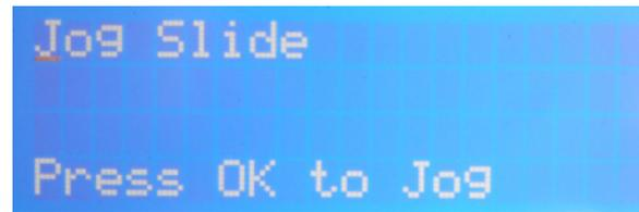
The next option on the AVHC is the **Jog Slide** screen. Pressing **OK** at this prompt will enable the torch to be manual toggled up and down the full range of travel. This is useful for positioning the torch but is not to be used when actually cutting. Once finished press **OK** again to exit the menu, be sure to not be in this menu while cutting as the torch will not fire when **Jog Slide** is enabled.
