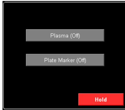
**MDI-** The Manual Data Input or MDI panel allows the execution or testing of g-code entered in the field. The g-code in the MDI field will override the currently loaded g-code file. Start will start the code entered here, reset will jump back to the beginning and hold will pause the code.
