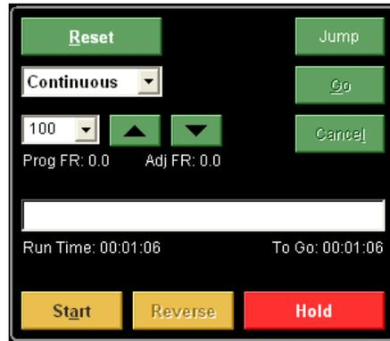
**Point-** Similar to the jog panel the point panel moves the machine for positioning. By typing in a coordinate in and pressing move the machine will travel that distance. A list of reference points allows quick movement to a particular point on the machine. The feed rate for the motion can also be set.
