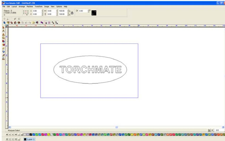
Once positioned go to 'Arrange' → 'Make Path'. What this function does is tell the CAD any overlapping part is a cut out of the main part.
