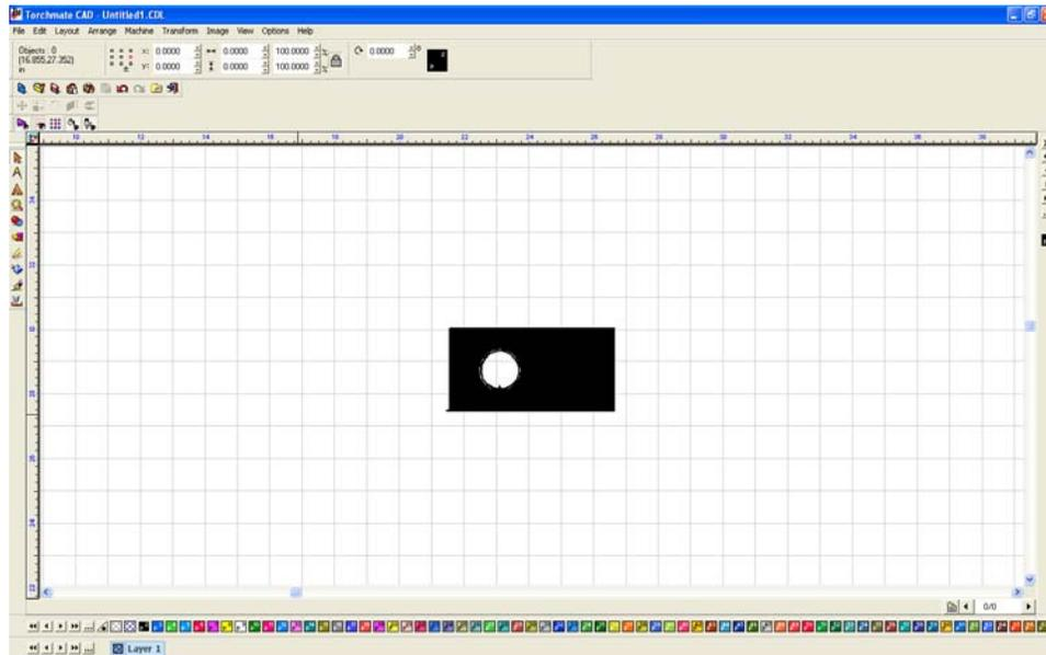
To eliminate the original drawing go to 'View' → 'Show Tool Paths' and ensure that it is unchecked.
