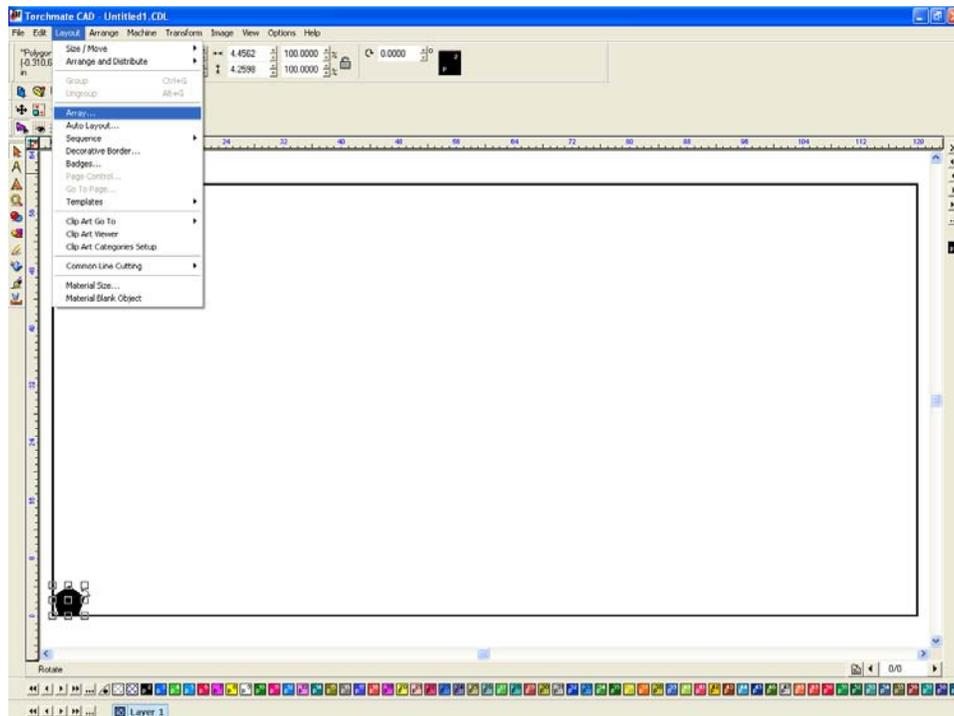
The array toolbar uses a pull down menu to select which type of array the CAD will create.
