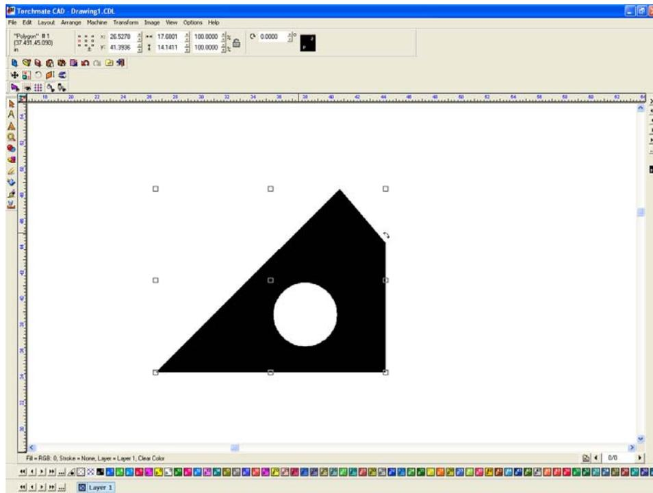
When importing DXF files keep in mind that some parts may have no issues while others can have several, it is always a good idea that before proceeding to cut or edit the part ensure that it is correctly imported.
