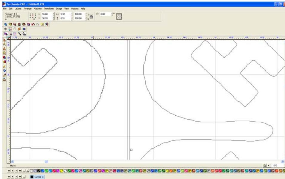
Once the ideal trace has been done the next step is to clean up any necessary defects. The first part of the process is to ungroup the trace so that each piece can be edited individually.
