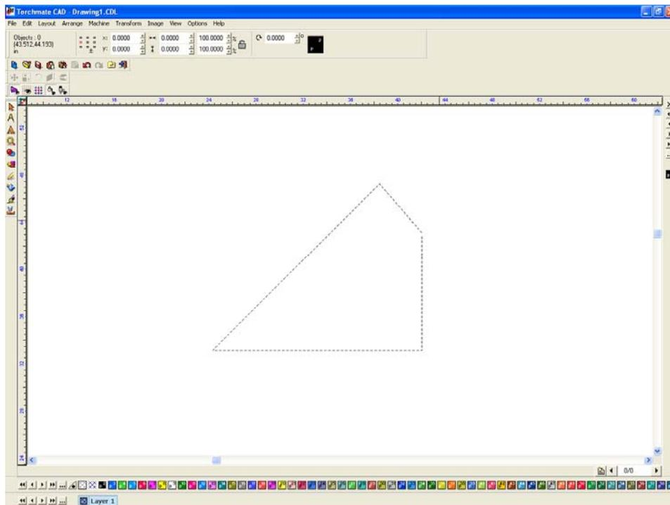
There are a few methods to try to correct this issue. The first method is to select the object go to 'Arrange' and select 'Connect Path'. The CAD will join any gaps within the prescribed gap tolerance.
