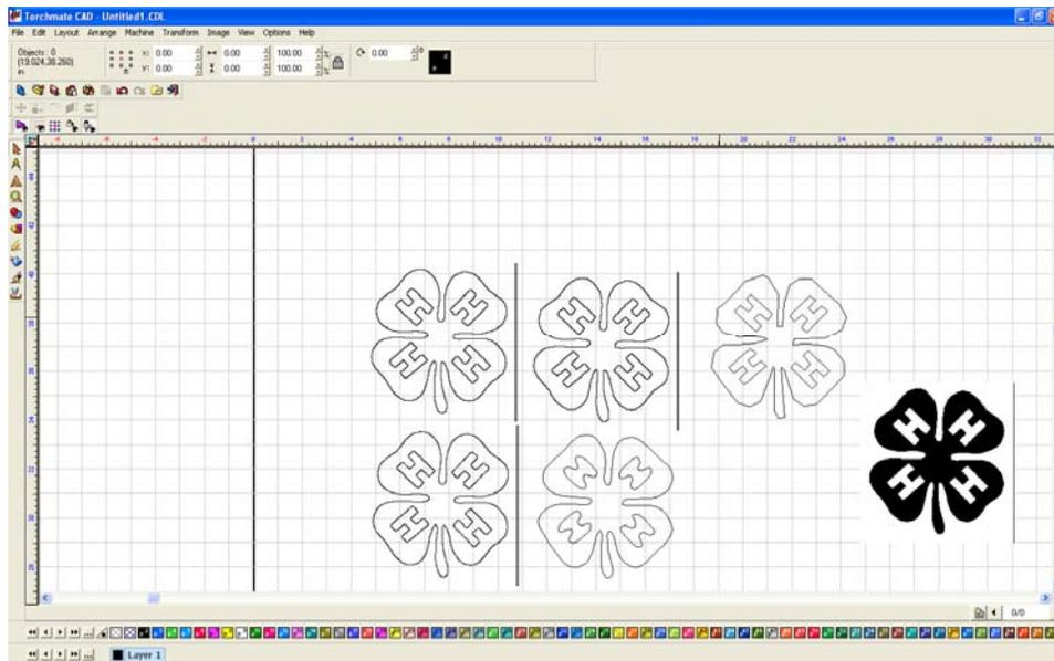
Zooming in reveals small subtleties of the two scans, the left scan is done with 10 and 10 as the line fit tolerances while the right image used 1 and 1.
