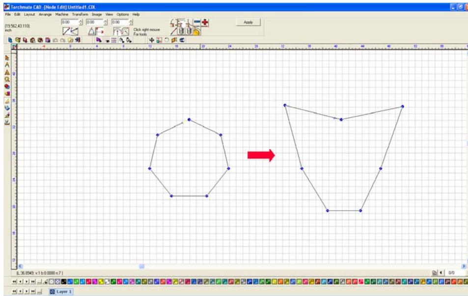
If the object is converted to curves or polyarc the edges can be changed into curves by hovering the mouse over the edge, it will appear as a hand. Clicking and dragging will adjust the curve.
