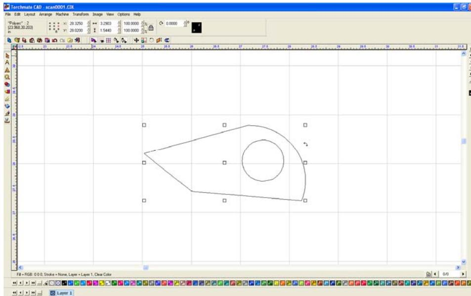
The traced object is now like any other object in Torchmate CAD it can be manipulated, added to, scaled, or tool pathed. To join the two objects as one go to 'Arrange' → 'Make Path'.
