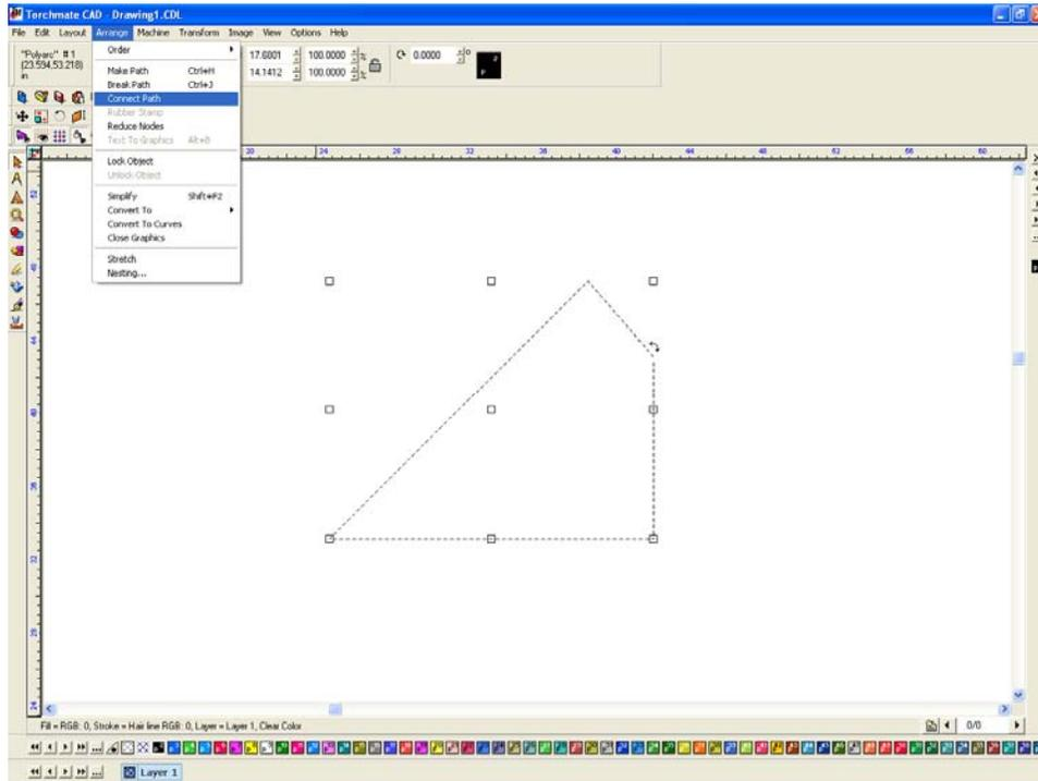
If connect path did not correct the gap the second method is to go into node editing. Double click on the object to enter node editing mode.
