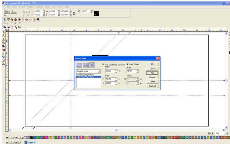
With diagonal lines an object can also be snapped to a corner, it will turn purple similar to an edge or the center.
