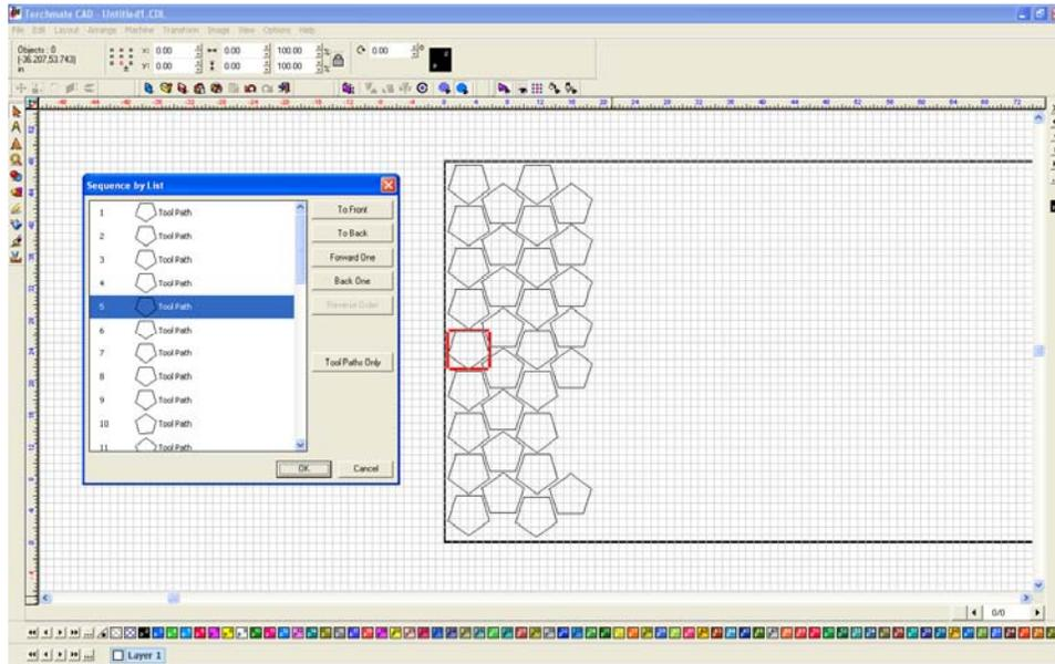
The order is changed by dragging a part up or down the list, or by using the positioning buttons in the menu.
