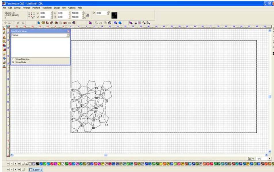
To change the order double click on any part, the 'To Position' window will appear. The number indicates the sequence position, simply type in the new position to change the order.
