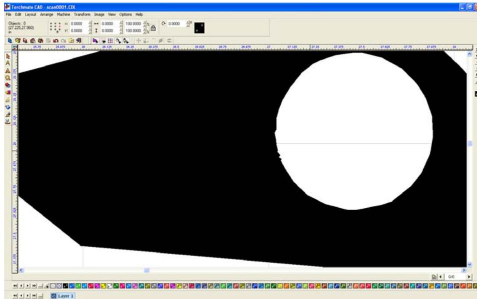
Begin by going to 'Arrange' → 'Break Path' this separates the hole from the outside part.
