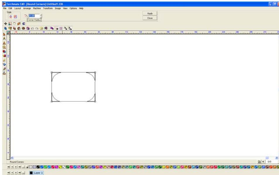
The rectangle tool also has sliding tabs that can create rounded corners. Select either of the tabs and slide to change the radius, there is also an entry box on the top tool bar that allows a specific radius to be set.
