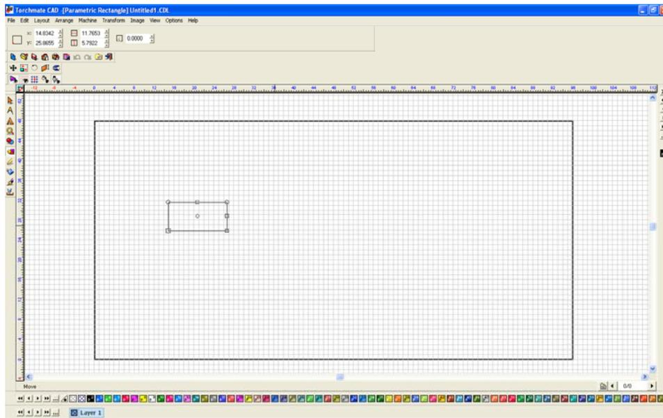
To change the rectangle's size select it by clicking on the edge of the part, then on the top tool bar type in the 'X' and 'Y' dimensions that are wanted and press enter.
