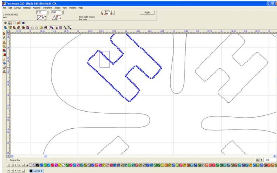
Once the letter is to a point where the only nodes left define the corners the letter may not look correct, almost ballooned sometimes. To correct this issue the nodes need to be changed. There are three types of nodes, a circle node is a rounded node, a cross is a sharp node, and a triangle is a tangent node. With a node selected, right click and move the mouse over the selection wanted and release.
