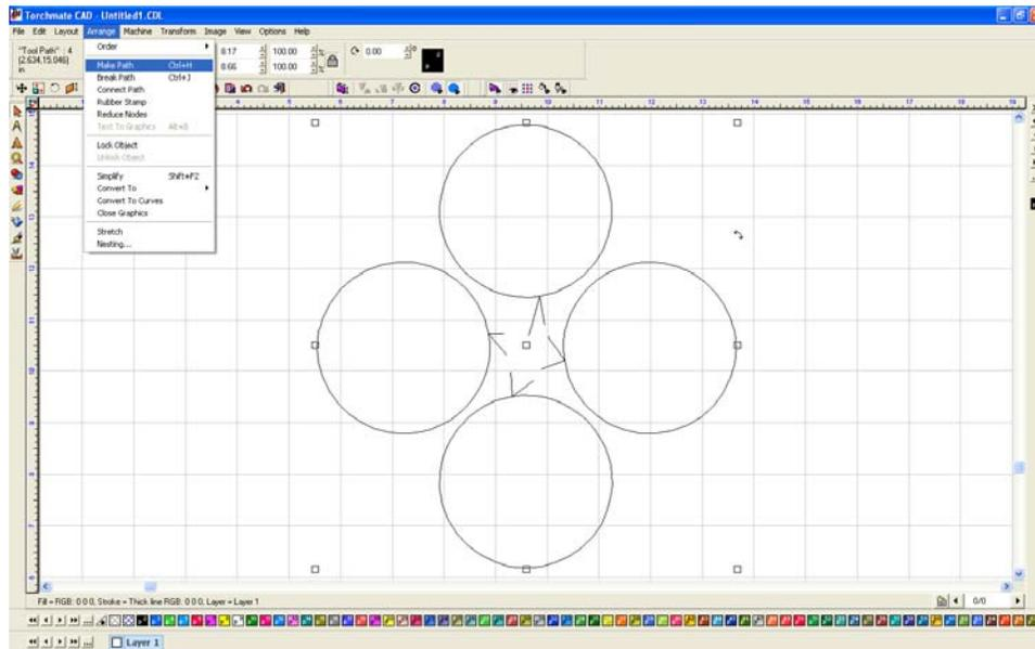
Double click on the parts to enter node editing. Join the lead in of one part to the lead out of another by selecting the two nodes, right-click, and select 'Join' (middle-top option).
