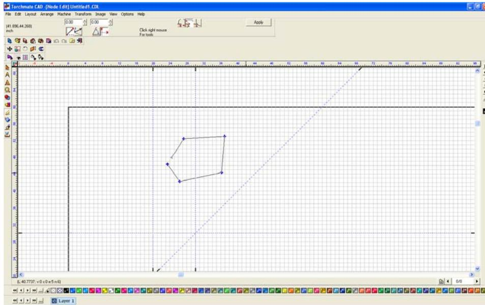
Nodes will snap to the guide lines when they are moved near them, this allows for multiple lines to be aligned to each other.
