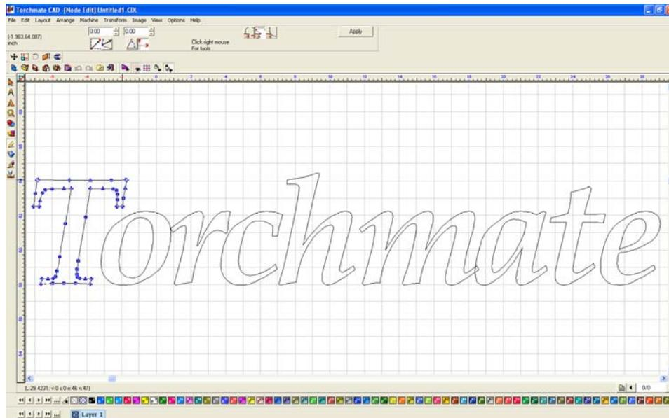
Unselected nodes are blue in color while a selected node will be red. To select a node click on it, or drag a selection box around a group of nodes. With a node or nodes selected they can be moved around.
