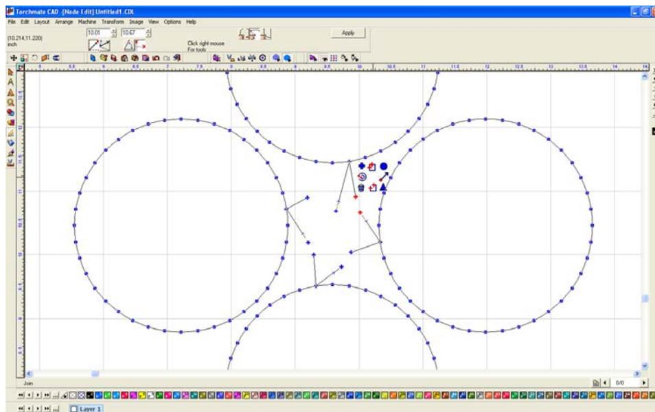
Repeat this with all of the parts leaving one lead in and one lead out not joined.
