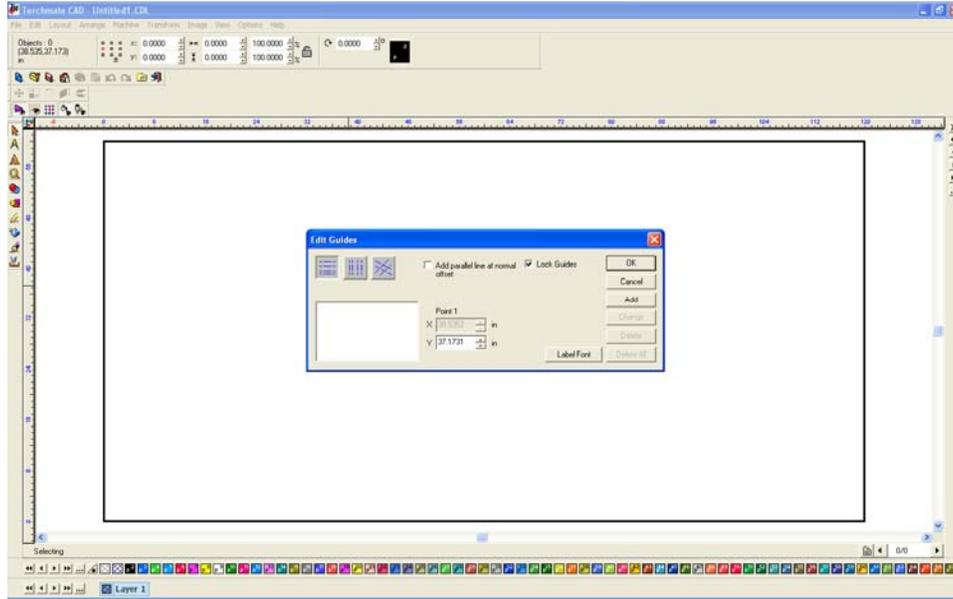
Guides use the coordinates related with the rulers. To add a line type in the coordinate the line will be at and select add. Horizontal, vertical, and diagonal lines can be added.
