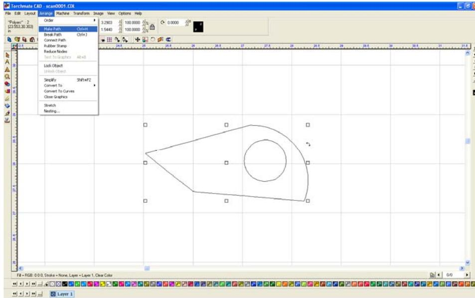
Just like any object 'Show Fill' from the 'View' menu displays how Torchmate Cad perceives the drawing.
