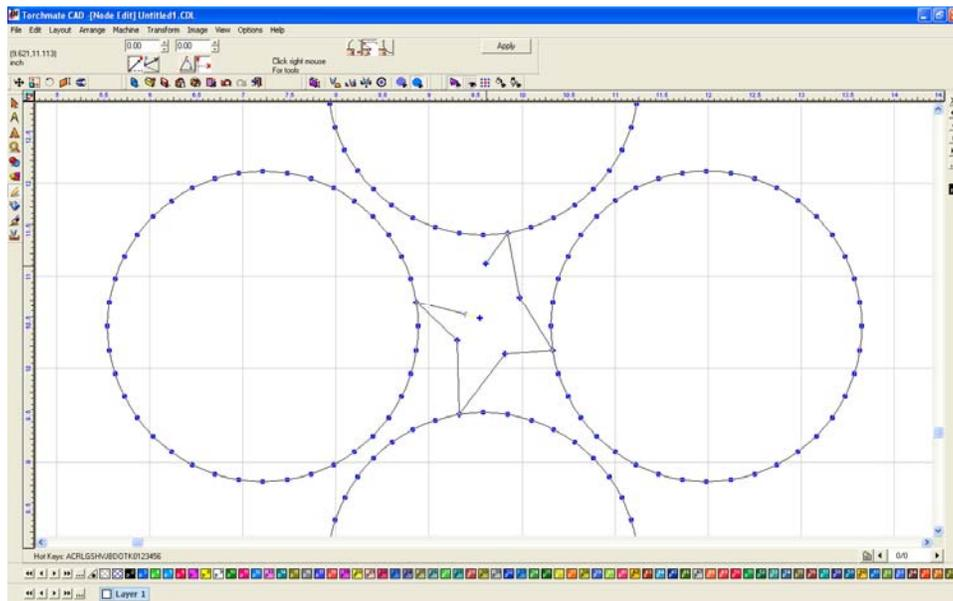
By joining the nodes occasionally the cut direction will change, to reverse it select the node that should be the starting point, right-click, and select 'Set Start Point' (the right-middle option).
