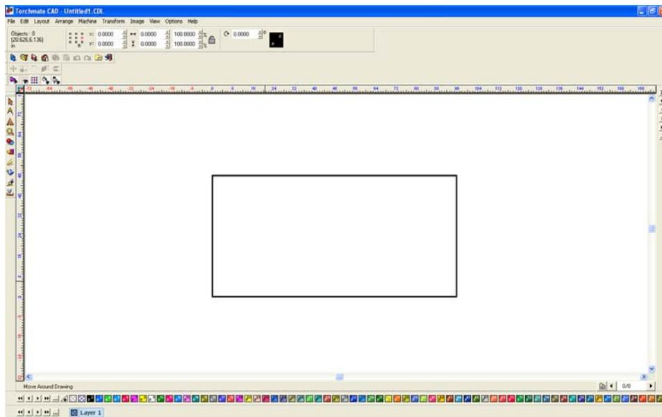
On the left-hand bar the shape tools can be accessed. The 'Shape Tools' menu has a few simple shapes to start most part drawings with (circle, oval, square, polygon, star, arrow and arch).
