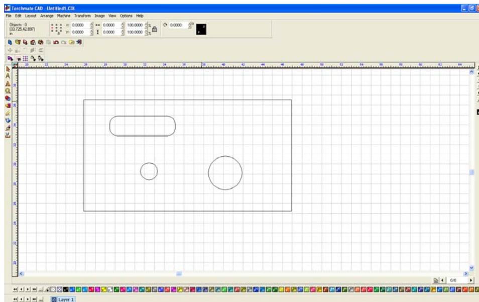
The part when it is just created is four separate objects the objects need to be merged together to one part. Select all objects that compose the part, then go to 'Arrange' and select 'Make Path'.
