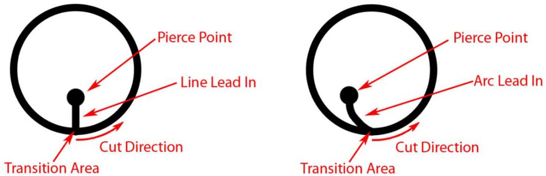
For a well calibrated table with minimal backlash a line lead in should be used, this will result in a cleaner transition area. The issue with an arc lead in occurs when the plasma's path comes around to finish the cut; it will encounter an area that has been partially cut on, and this can result in a divot or excess slag forming in the transition area. In outside cuts or non-circle inside cuts the lead in type generally will make no difference to the final quality.
