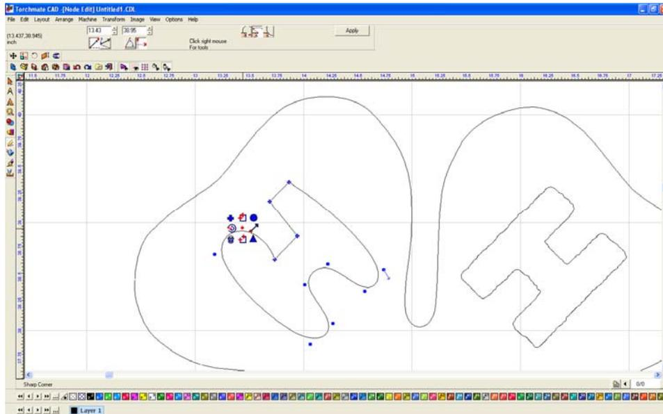
Once the nodes are squared reposition the nodes by selecting one and moving it. Once all the nodes are in the correct position press the apply button.
