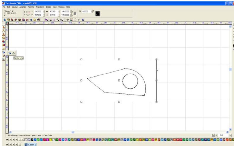
The 'Tracing Setup' for center line scanning is similar to accuscan's. Tolerance will adjust how tightly the image is followed; corner sensitivity will affect how close corners are cut.
