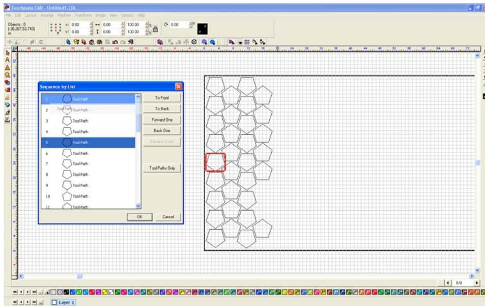
Any time the cut order is changed it can be viewed again by going to the 'Tool Path Viewer' in the 'View' menu. Keep in mind that the order displays a part with multiple cuts simply as a single number.
