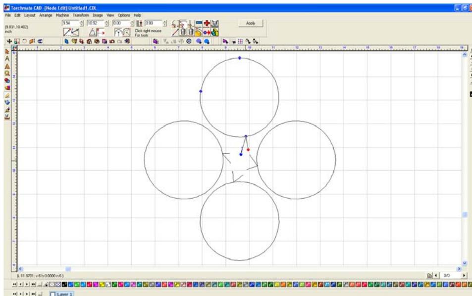
Select all of the tool paths, go to 'Arrange' → 'Make Path'. This converts the tool path back to a polygon but allows the parts to be joined together.
