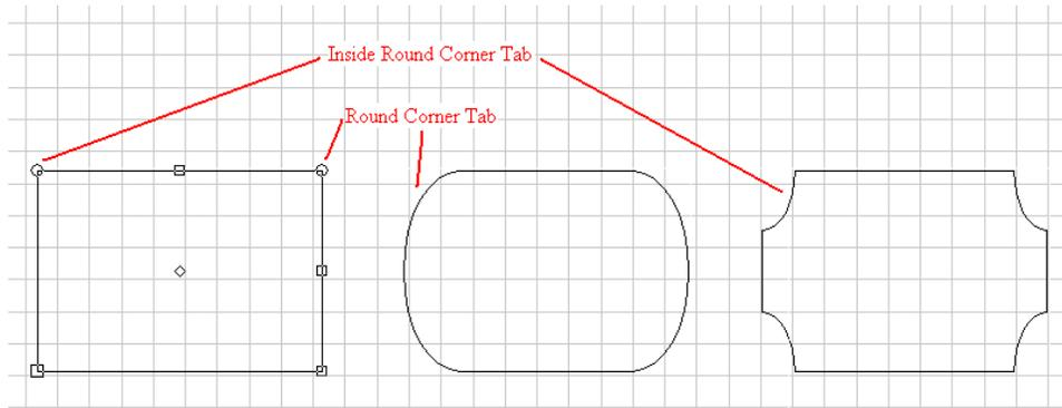
'Round Corner' rounds all four corners of a square. In order to round one corner at a time, or to round corners on non-square shapes use the 'Fillet Round Corner'.
