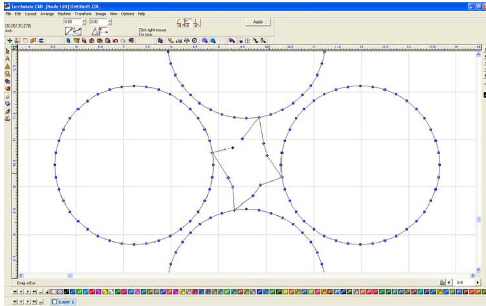
The nodes can be edited just as any drawing and the leads can be cleaned up by eliminating some of the nodes.
