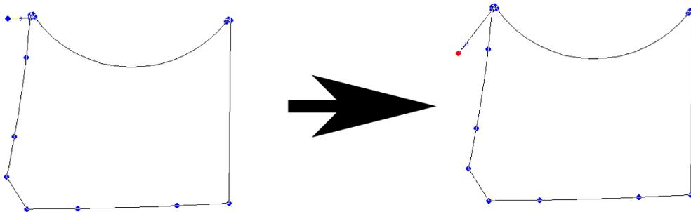
The point where the lead in connects to the part can also be adjusted after the tool path is made. When the tool path is selected and in node editing mode (by double clicking on the tool path) the top tool bar will have twelve small boxes, one of them adjusts the start point. Simply select the start point tool and click on the part where the new start point should be.
