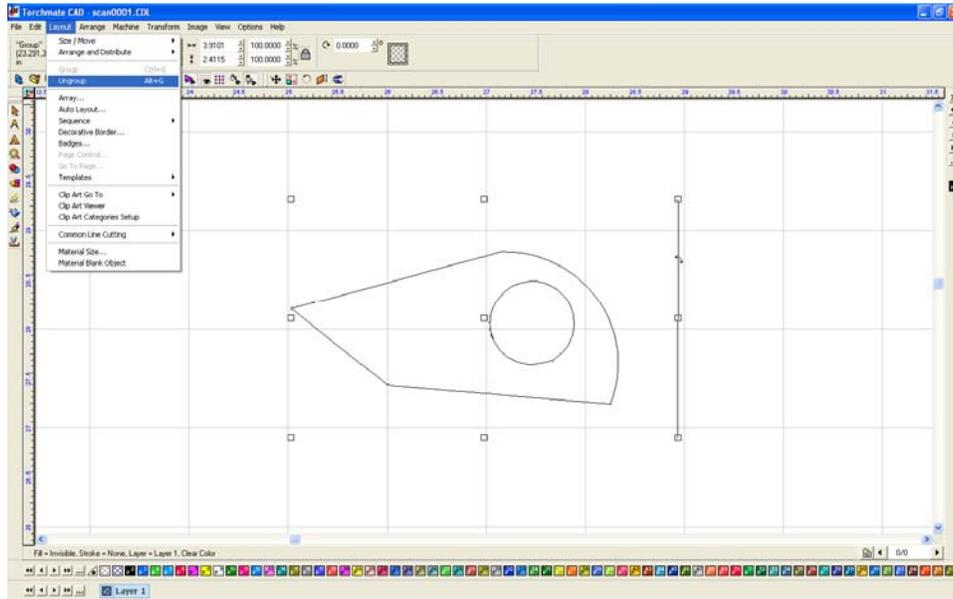
Depending on the quality of the trace the image may be in multiple parts, Torchmate CAD indicates how many objects selected in the upper left corner of the toolbars.
