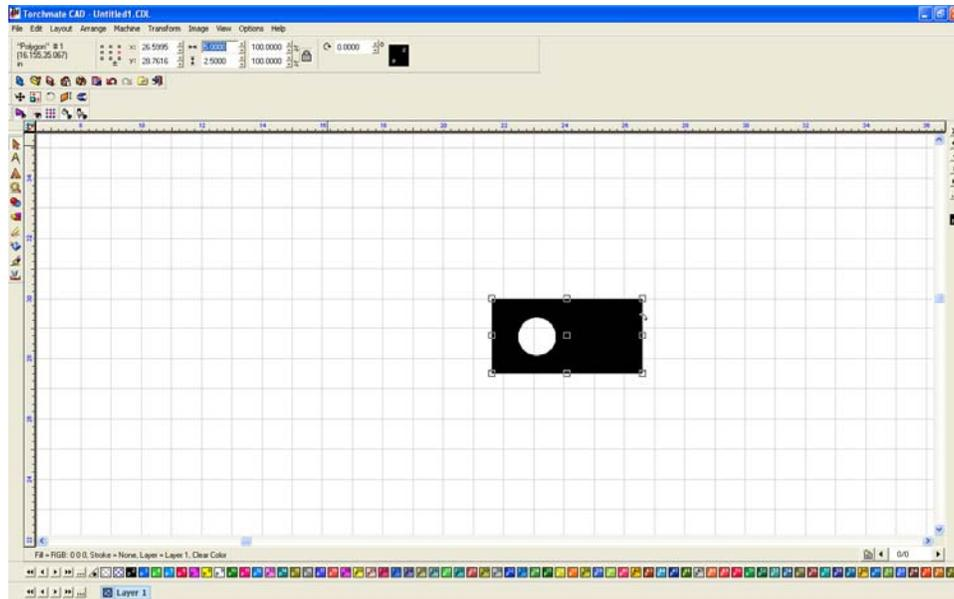
If the part is the correct size and 'Show Fill' appears correct the part is ready to have a tool path created.
