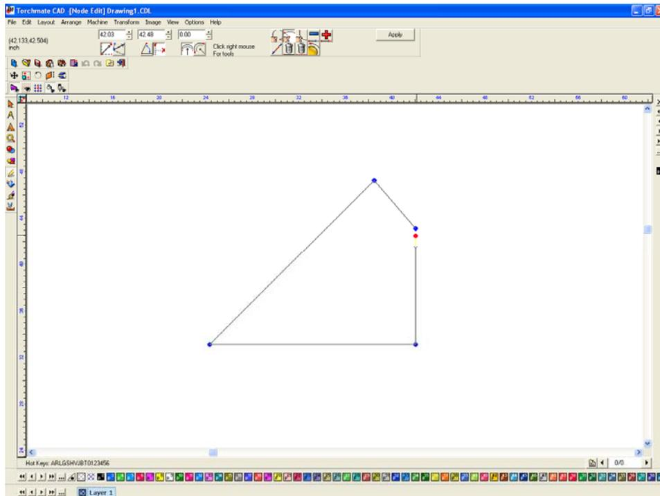
Select any node and it will turn red. If the 'Tab' key is held down the CAD will cycle through the nodes selecting each one in sequence. If there is a gap the cycle will stop and pressing 'Tab' will do nothing. At any place there is a gap select the node, hold down right-click, this brings up the node options. The top middle option is join this will join the node with a nearby un-joined node. Verify with 'Show Fill' that the part corrected.
