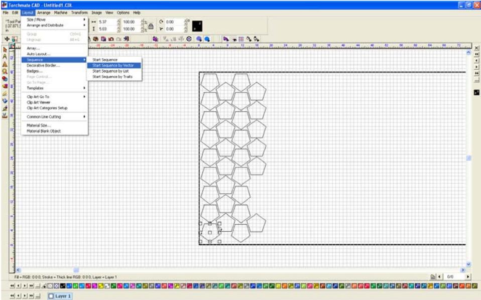
With ‘Start Sequence by Vector’ it is not necessary to click on each part to order them, simply by clicking on two parts will also order the parts in-between in series. This is useful for rowed parts since only the parts on the end of the rows need to be clicked to sequence the entire sheet.
