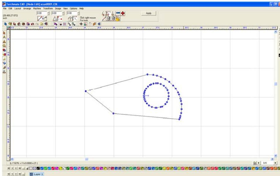
If a hole comes out jagged from the trace node ending can be time consuming. In some cases the easiest option is to redraw the hole with the circle tool.
