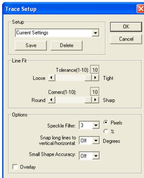
Once the trace setup is done clicking on the vectorization button creates the line trace. There are now two objects on top of one another. Moving one off to the side the two can be compared.
