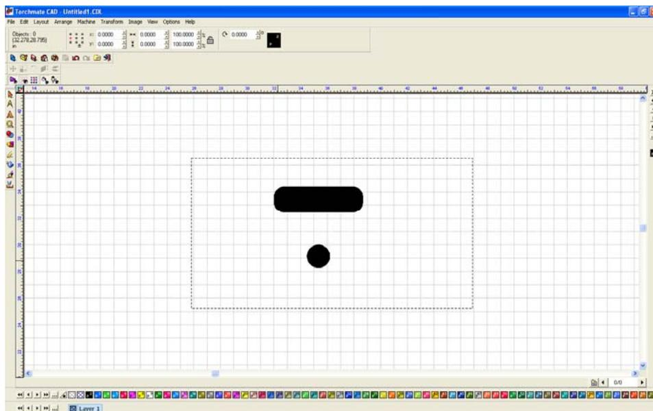
Select the object and choose 'Connect Path' from the 'Arrange' menu. The CAD will ask for an 'Allowable Error' this is the maximum distance it will attempt to join a gap.
