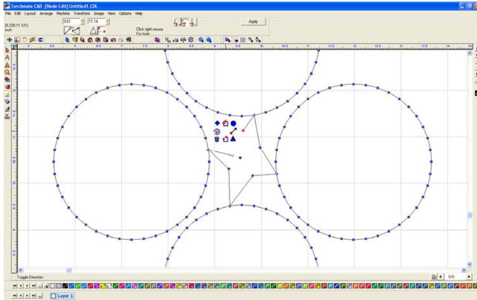
The parts are now joined; the last step is to create a tool path again. This time the tool path will be 'Online' since the offset was already done the first time the tool paths were created.
