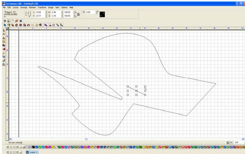
Nodes can also be used to edit existing shapes, even shapes that are created with shape tools. For any shape created with the shape tools there is one step that must be done to be able to node edit. With the part selected go to 'Arrange' and 'Convert To' select either 'Polygon' or 'Polyarc'. Double clicking on the object will now bring up node editing. The process of converting will not allow the part to be edited further by the shape specific tool bar.
