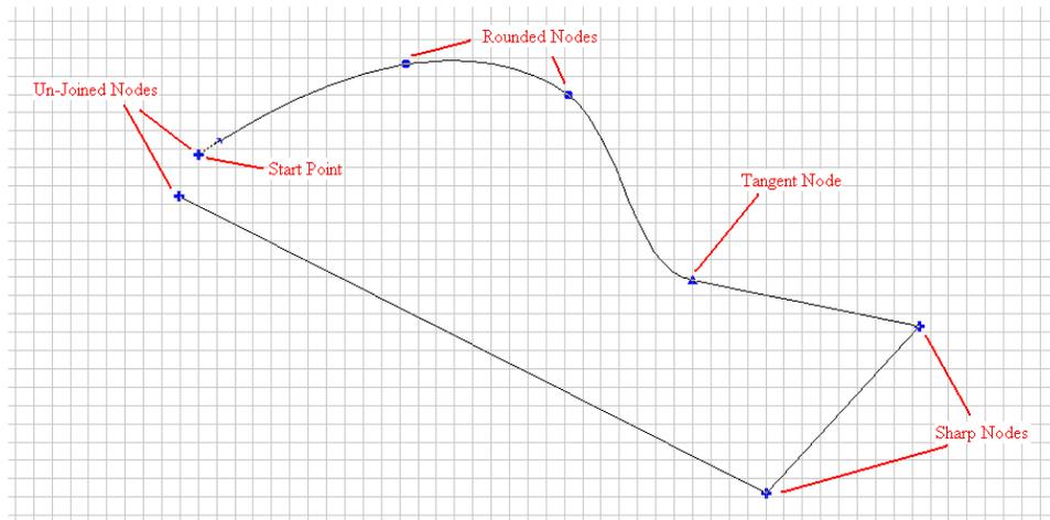
When a node is selected additional features can be accessed by right clicking and holding. Depending on the image type there will be up to eight options. Move the mouse over the option desired and release the right mouse button, this will select the option highlighted.
