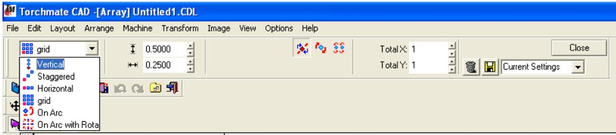
Grid, vertical, staggered, or horizontal all work on the same principle. The tool options allow for spacing along each axis as well as how many copies are desired.
