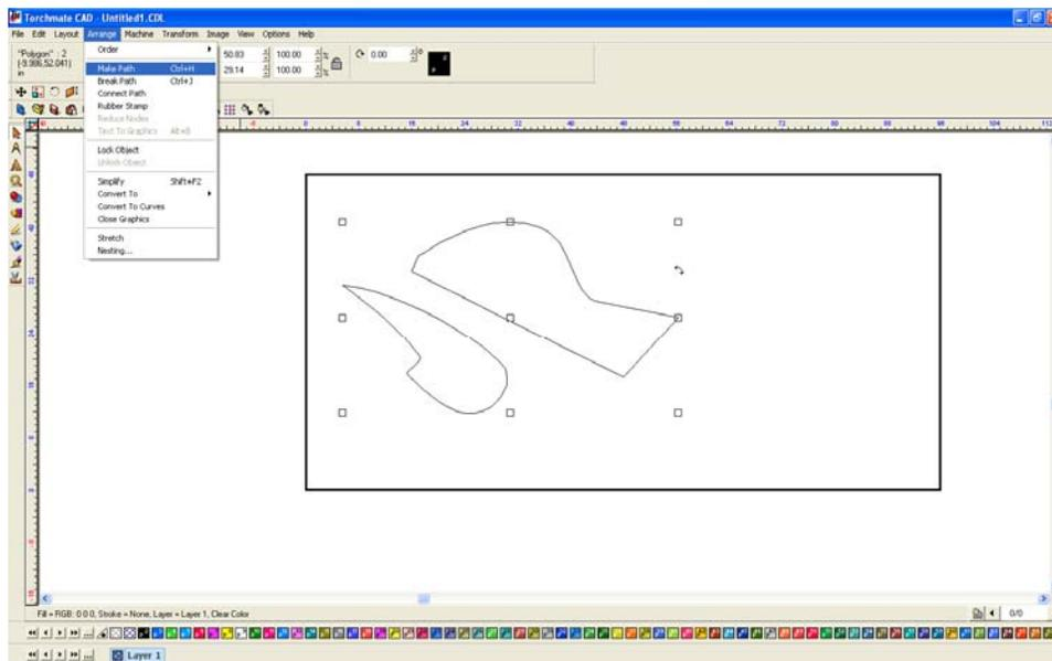
With the paths joined the next step is to edit the nodes to create a bridge between the parts.
