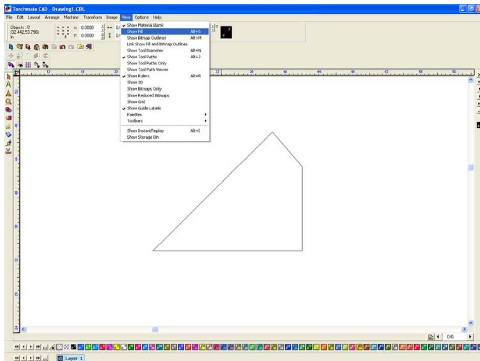
Show fill displays the object as the computer sees it. If the object is filled in solid then it is ready to have a toolpath created.
