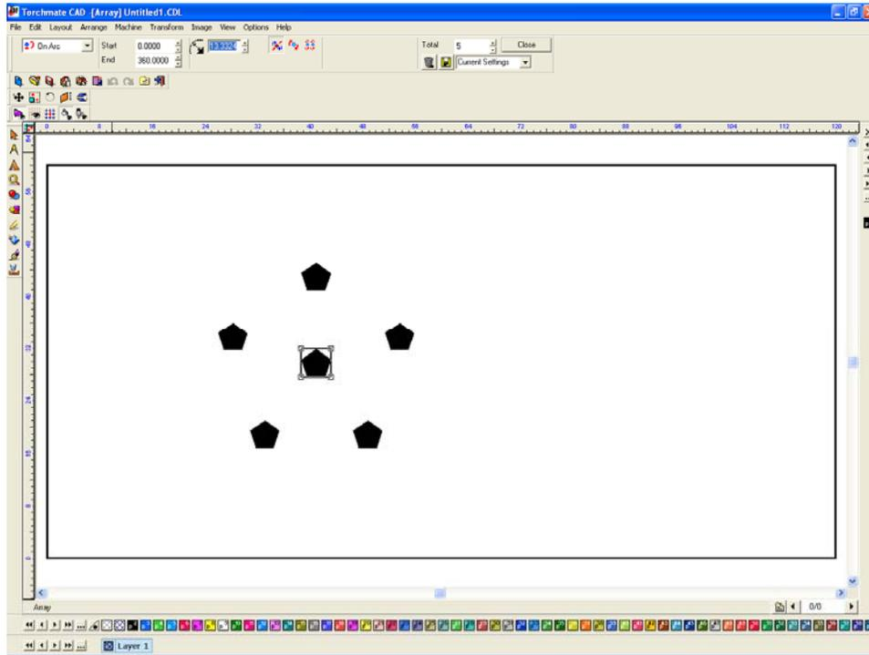
‘On Arc with Rotation’ creates the duplicates around the original equally spaced as the ‘On Arc’ does, but it will also ensure that the part’s base is facing toward the center.
