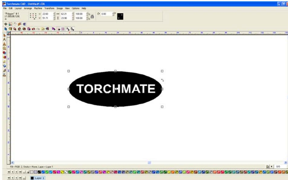
To bridge a letter simply draw a small rectangle over the area wanted to be bridged and complete a 'Basic Weld' from the weld menu on the left hand toolbar.
