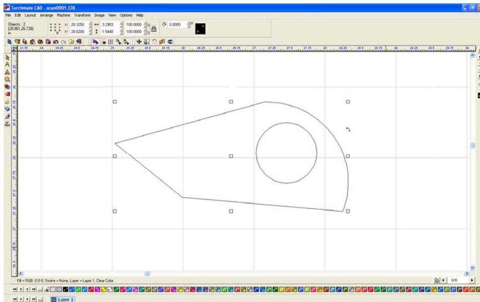
Just as before the objects can be made into one part by going to 'Arrange' → 'Make Path'.
