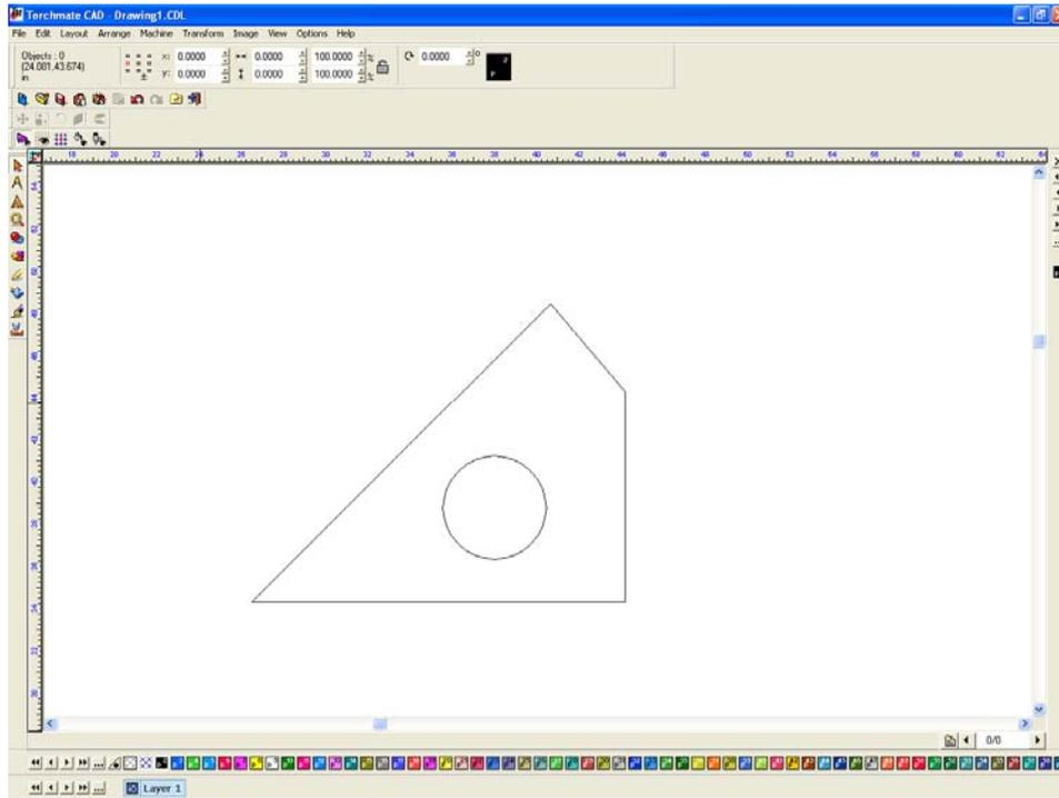
In this case the fill displays each object as solid, the CAD simply does not associate the hole with the rest of the part.
