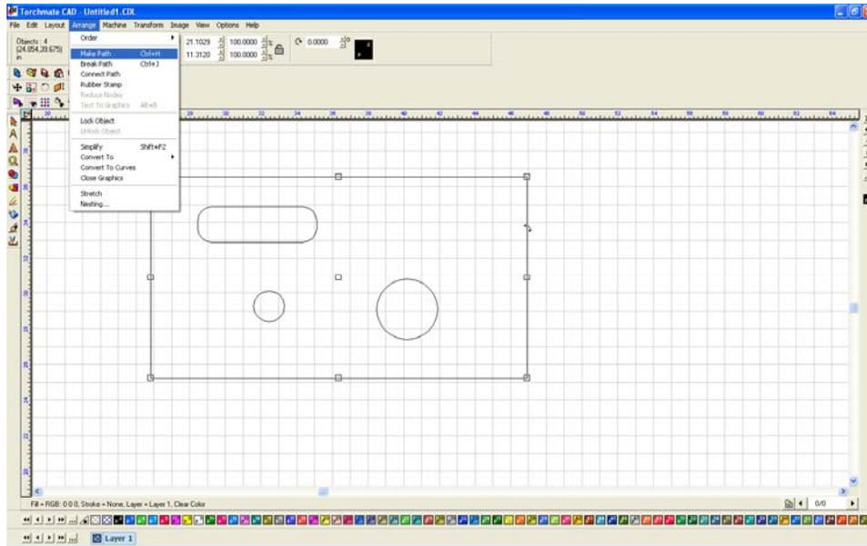
The objects are now one part and one path. The best way to ensure that this is the case is to go to 'View' and select 'Show Fill' this displays the object as the CAD interprets it; the filled in parts indicating the actual part.
