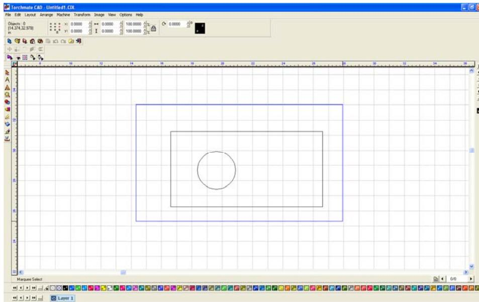
With both objects selected go to ‘Arrange’ → ‘Make Path’. This option tells the CAD that all objects selected are one part, allowing the software to determine if something is a hole or cutout.
