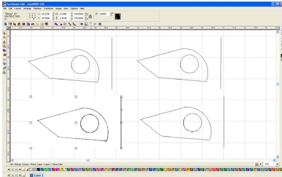
When a trace is done with center line scanning the resulting image will be grouped together. The first step in editing the image is to go to 'Layout' → 'Ungroup'.
