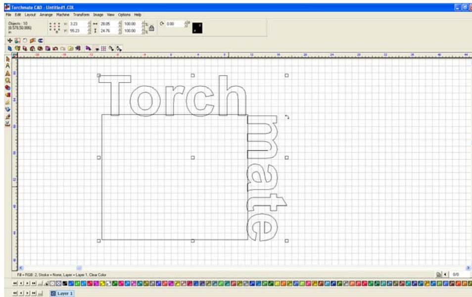
Here is a combination of manipulating text along a path and cutting out text.
