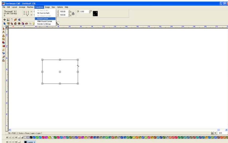
When 'Round Corners' is enabled the top menu will have a dialogue box that allows the radius to be specified.
