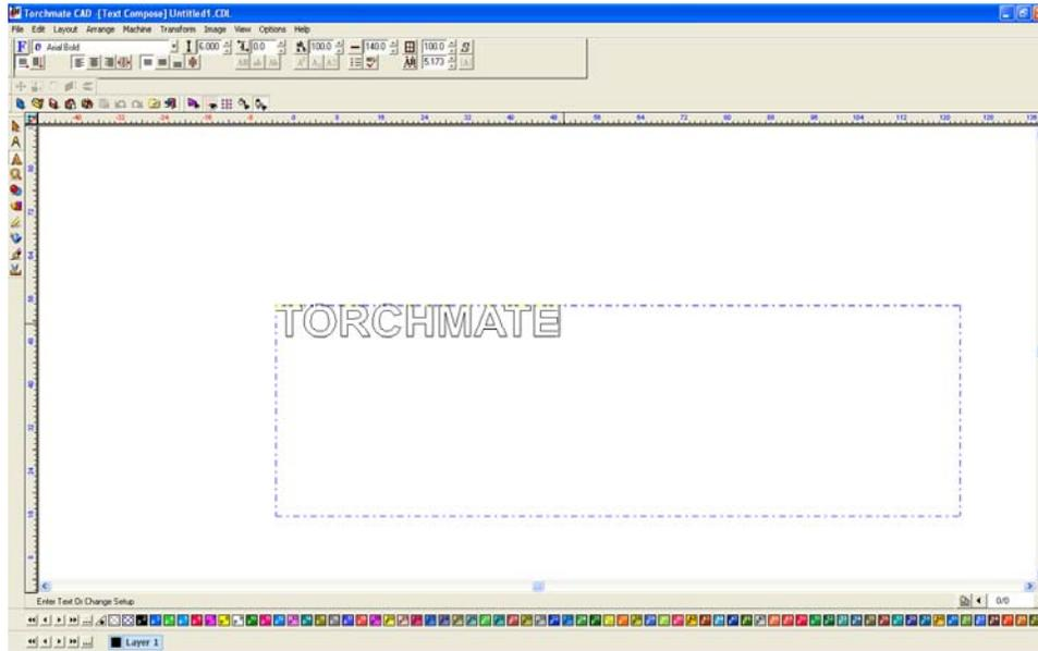
Once satisfied with the text in order to edit the text further it must be converted to a graphic. With the text selected go to 'Arrange' → 'Text to Graphics'. The letters are now individually selectable and can be manipulated as any other drawing. Examples below illustrate some basics of what can be done.
