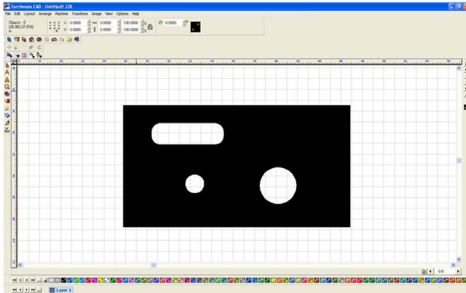
The object is now a single part that can be moved around, all of the nodes can be edited at once as well. To edit a single hole or the outline without changing any parts use break path the separate the objects back to individual elements. Any element can now be changed. Once changed select all parts and 'Make Path' again to revert the objects to a single part.
