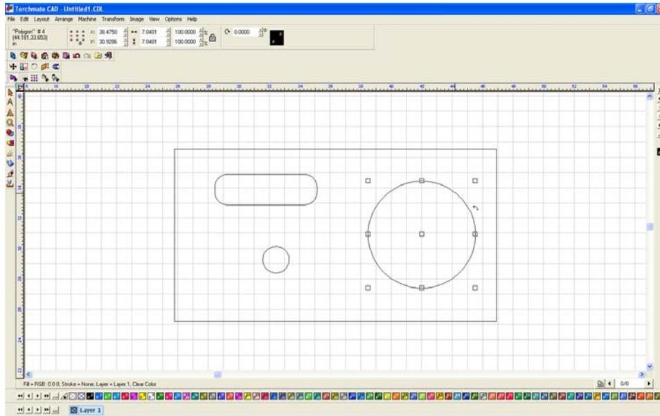
Using 'make' and 'break' path allows for the editing of single components of a part or the merging of elements to create a part. Show fill is an invaluable tool for keeping track as to what stage a part is in as it will show what the computer is considering a part.
