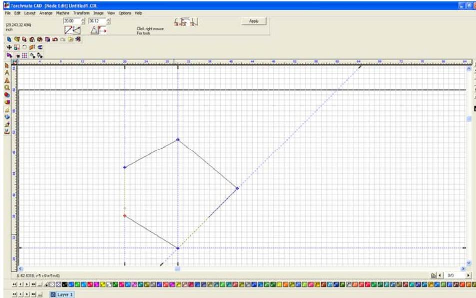
Another way of aligning objects is to go to 'Options' select 'Grid' and then 'Snap to grid' with this option enabled the object's edge will attempt to align with the nearest grid line.
