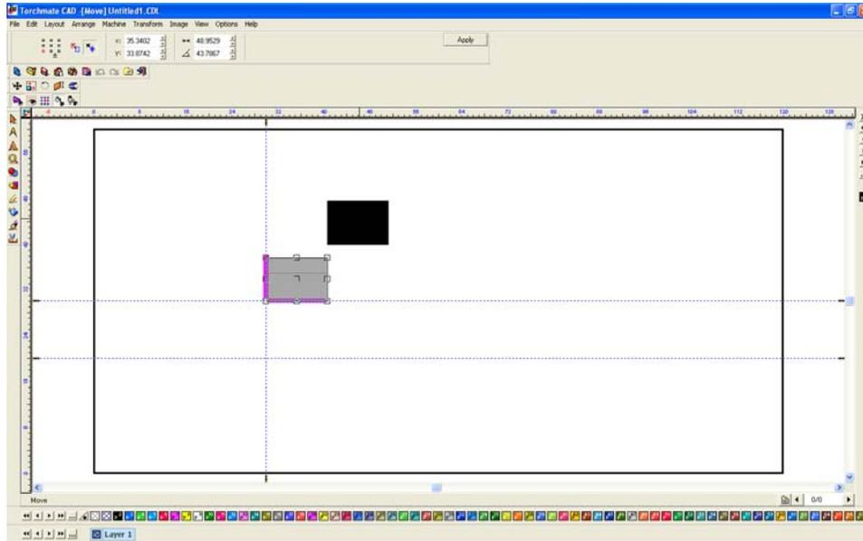
Objects can be snapped to any edge as well as to the center line of the object.
