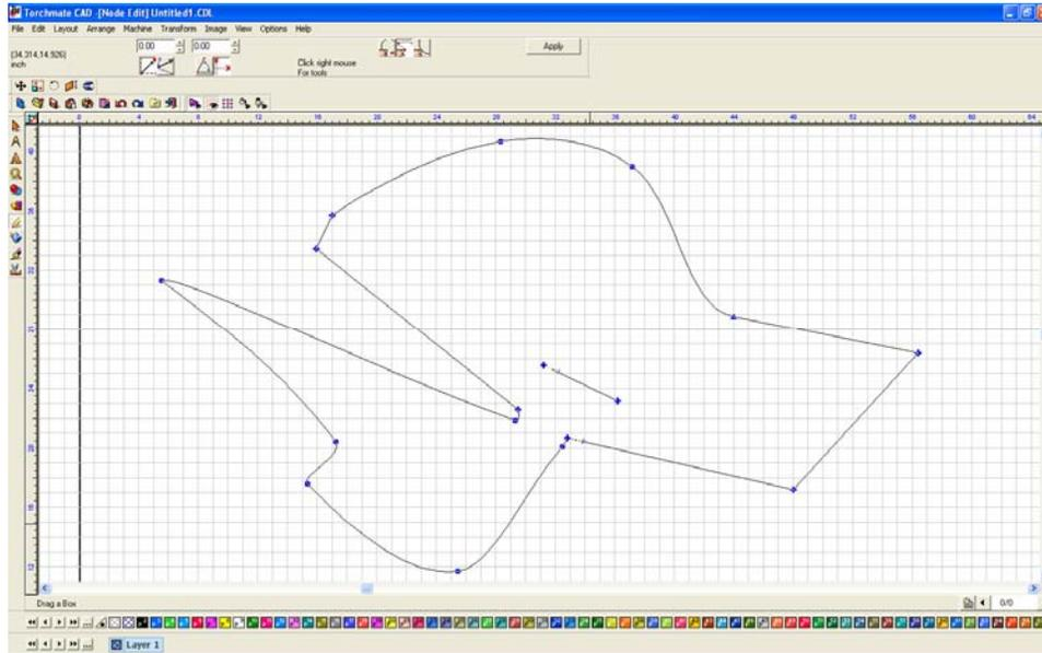
If the shape is more complex the way to delete the scrap is to break the path. Select the part and go to 'Arrange' and 'Break Path'. This separates any un-joined parts into distinct objects.
