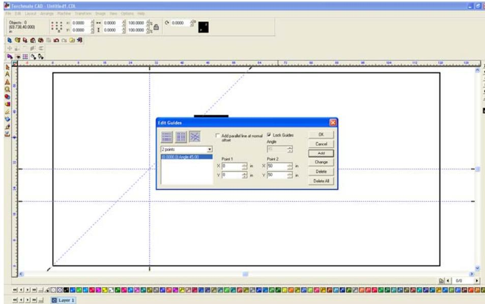
Any line can be added parallel to an existing line by selecting the ‘Add parallel line at normal offset’ check box. A new box will appear to enter how much of an offset should be used.
