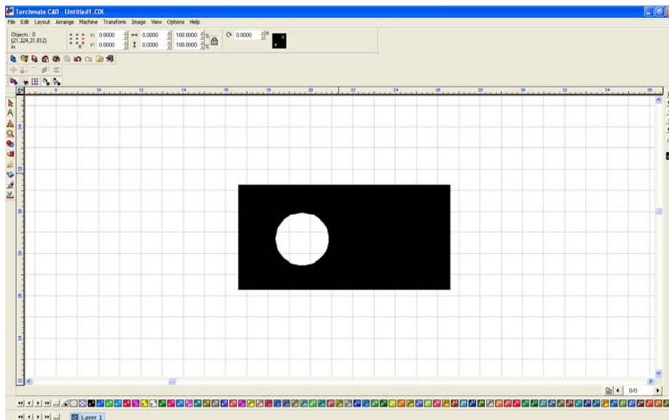
Once the part is finished it can be resized again if necessary, this resizing will adjust the hole's size along with the part's size.
