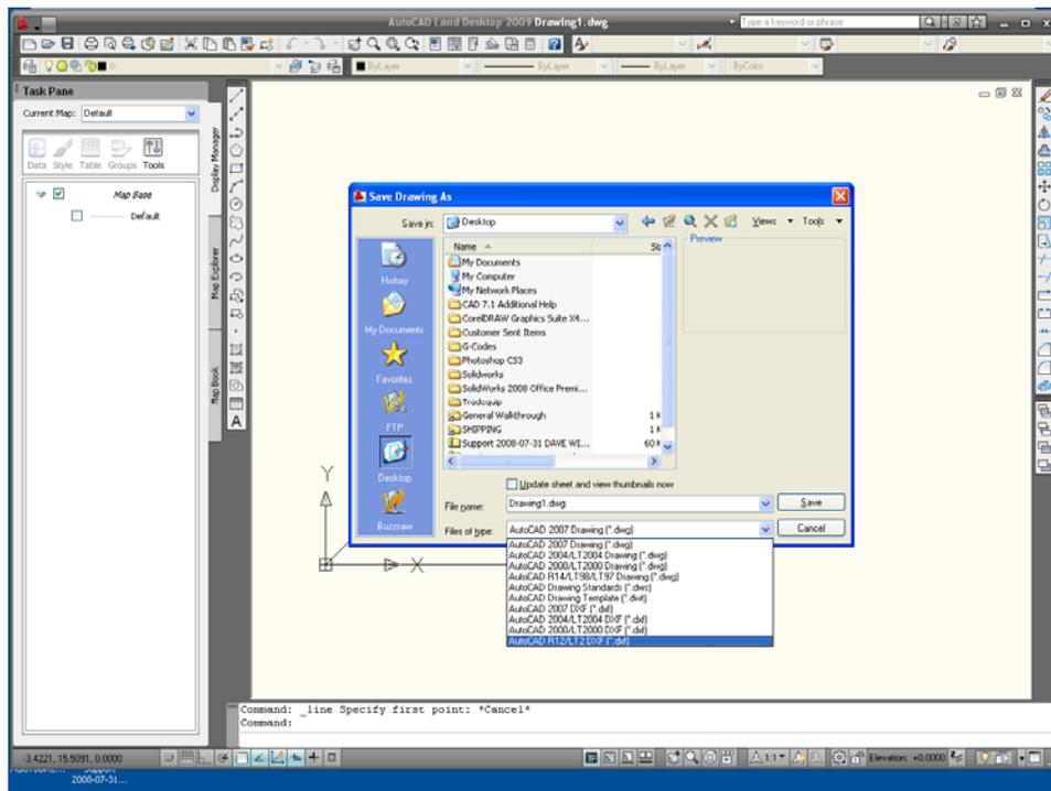
Now that the DXF is saved go into Torchmate CAD, go to 'File' and select 'Import'.
