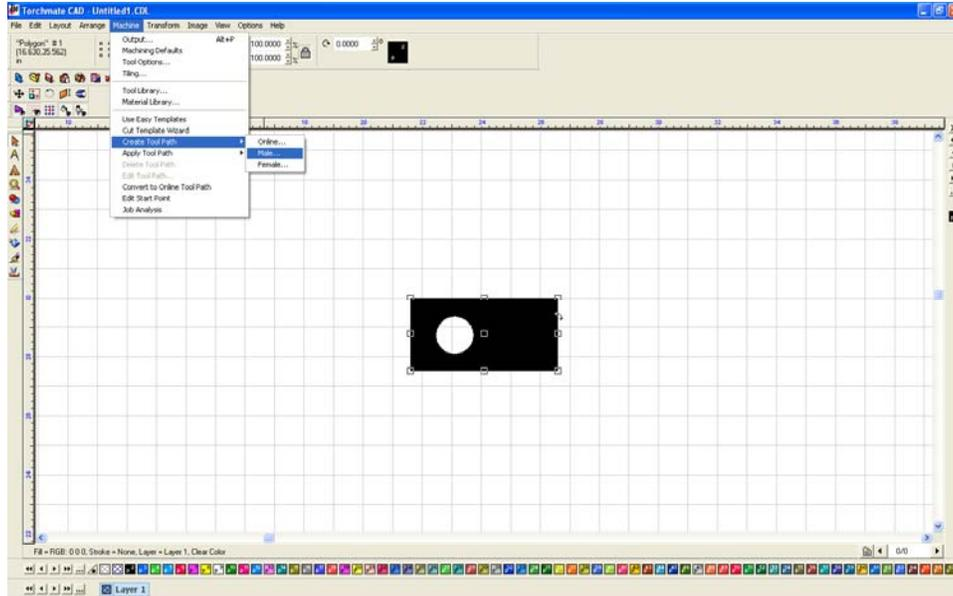
For this simple part the only changes to be made are under the 'Lead In/Out' tab. Create a lead in by specifying a length and angle. Then press 'OK' to create the tool path.
