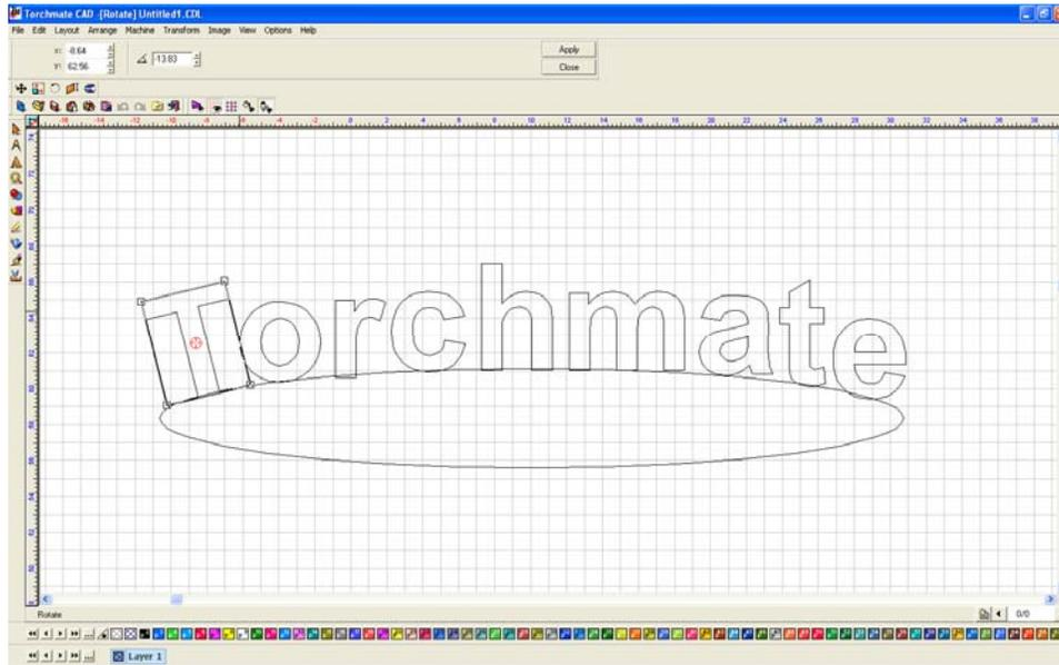
Once all the letters are rotated, delete the arc if it is not needed. This process can be done with shapes as well as arcs, or any shape desired.
