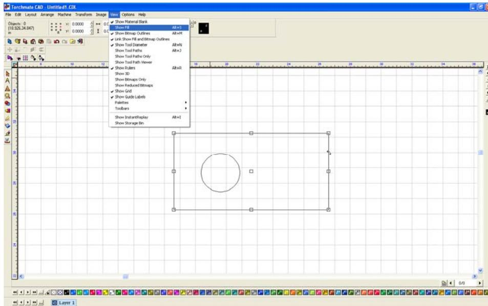
With 'Show Fill' on the part will fill in what is perceived as the part. Holes should be empty with the metal part filled in.
