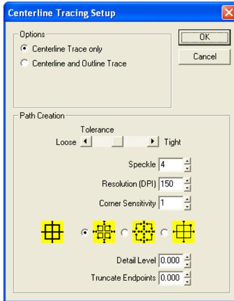
As before multiple scans can be done slightly changing the settings. This method allows for side by side comparison of trace settings to find the ideal one for the particular scan.
