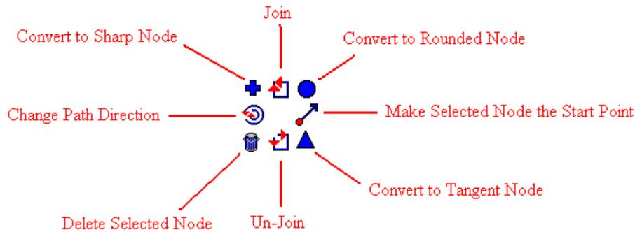
Node editing can be used to join two unrelated objects together. To get into node editing for a shape double click on it. Initially the two objects can be edited but not at the same time.
