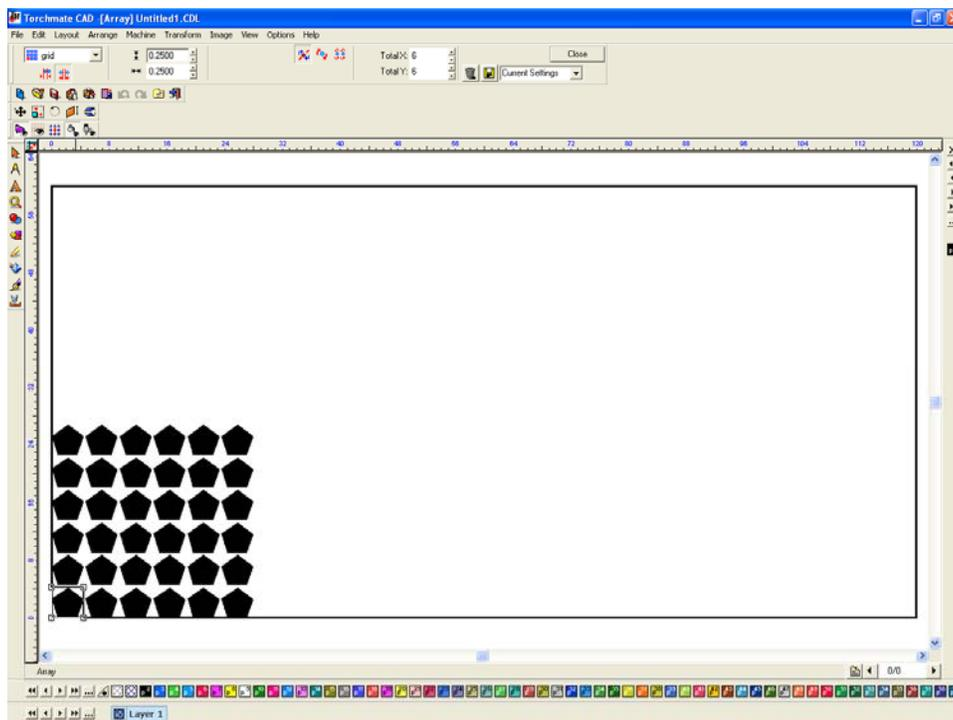
‘On Arc’ arrays specify how many copies and a distance from the center, the parts are then arranged equally around the original part equally spaced.
