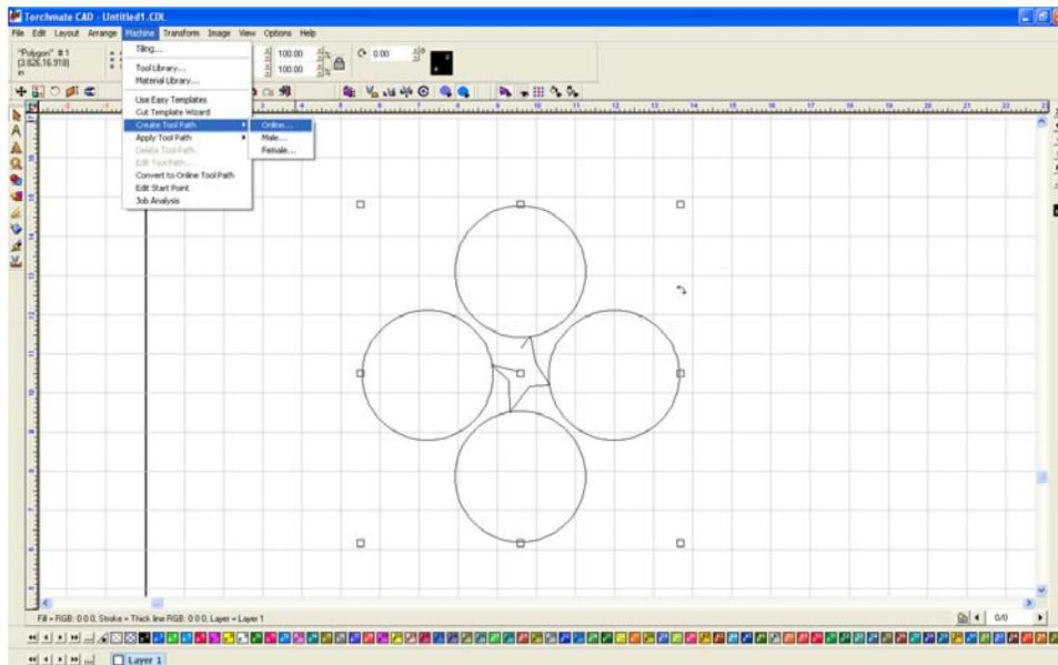
Again keep in mind when using common line cutting with plasma cutting the plasma can go out when traveling over an already cut area. When cutting parts with holes the holes will need to be created separately and cut order will have to be edited before cutting.
