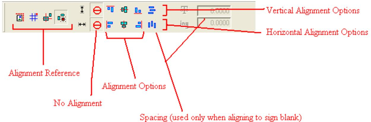
The alignment reference area specifies what the objects are being aligned to.
