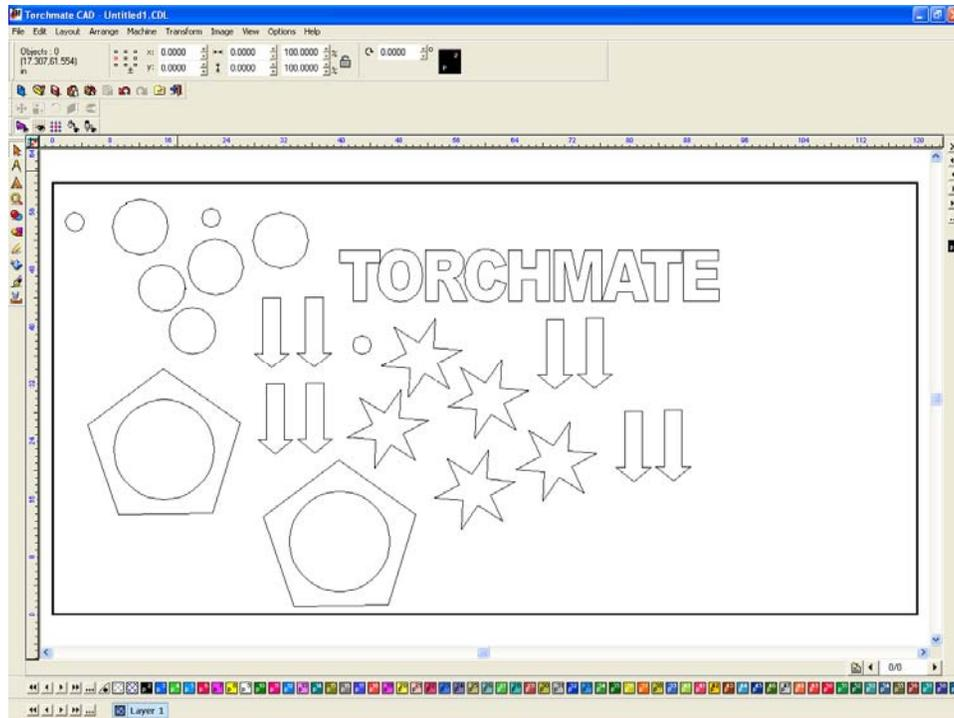
The nesting feature uses a defined material size as its guide to arranging parts.
