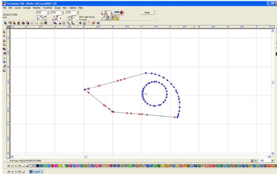
The outside part is now cleaned up, the inside hole can also be cleaned up in node editing.
