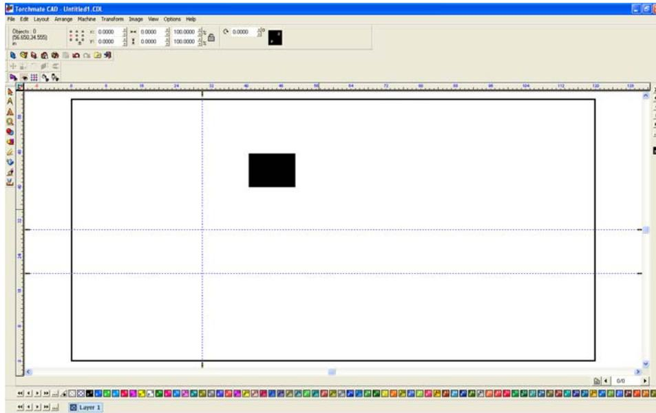
To snap an object to the guides move the object over to the guides, when the edge of an object turns purple the object is aligned to the guide.
