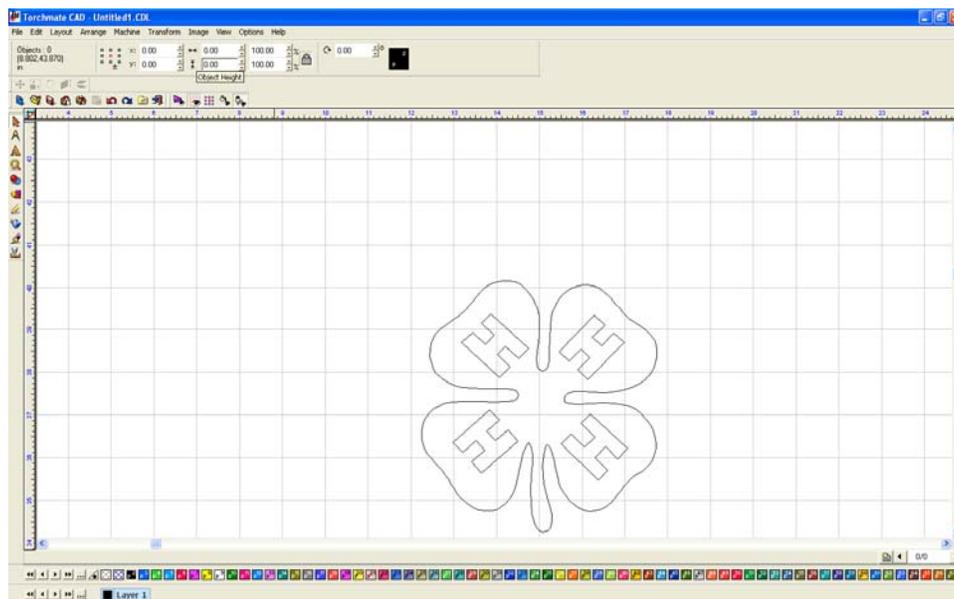
Select 'show fill' from the 'view' menu, the CAD software is now displaying the object as it sees it. In this case the object is not correct as the letters are not visible.
