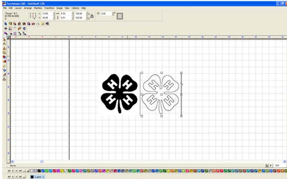
Repeating vectorization multiple times with different trace setups allows the comparison of settings in order to determine the best one for a particular image. Each image brought in may have different trace setups based on the quality of drawing and scan.
