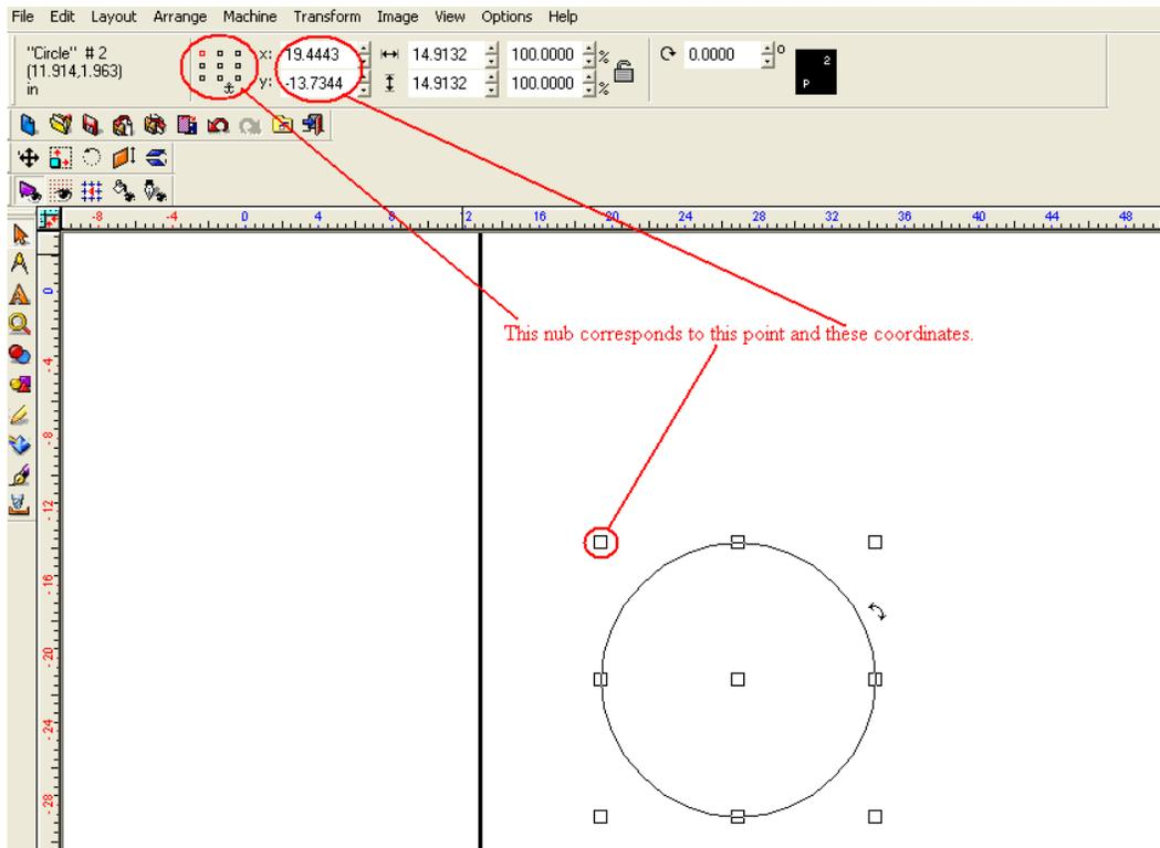
Using the alignment nubs two points on two objects can be aligned to the same coordinates simply by changing the coordinates in the boxes.
