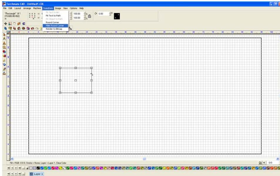
A similar toolbar will appear on the top. In order to specify which corner or angle to be rounded click on the corner, when done click apply then close. The 'Fillet Round Corner' tool can be used multiple times to make various radii sizes on different corners.
