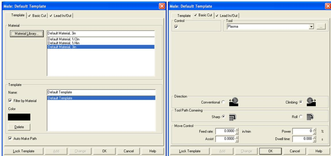
If this tab is used what it stores is the information from the other two tabs as a material. For instance the settings can be set for one thickness, once the settings are made selecting change on the bottom row of buttons updates the selected material so that in the future the settings load with the specific material. Again if nothing is ever changed on this page the tool paths will never be affected.
