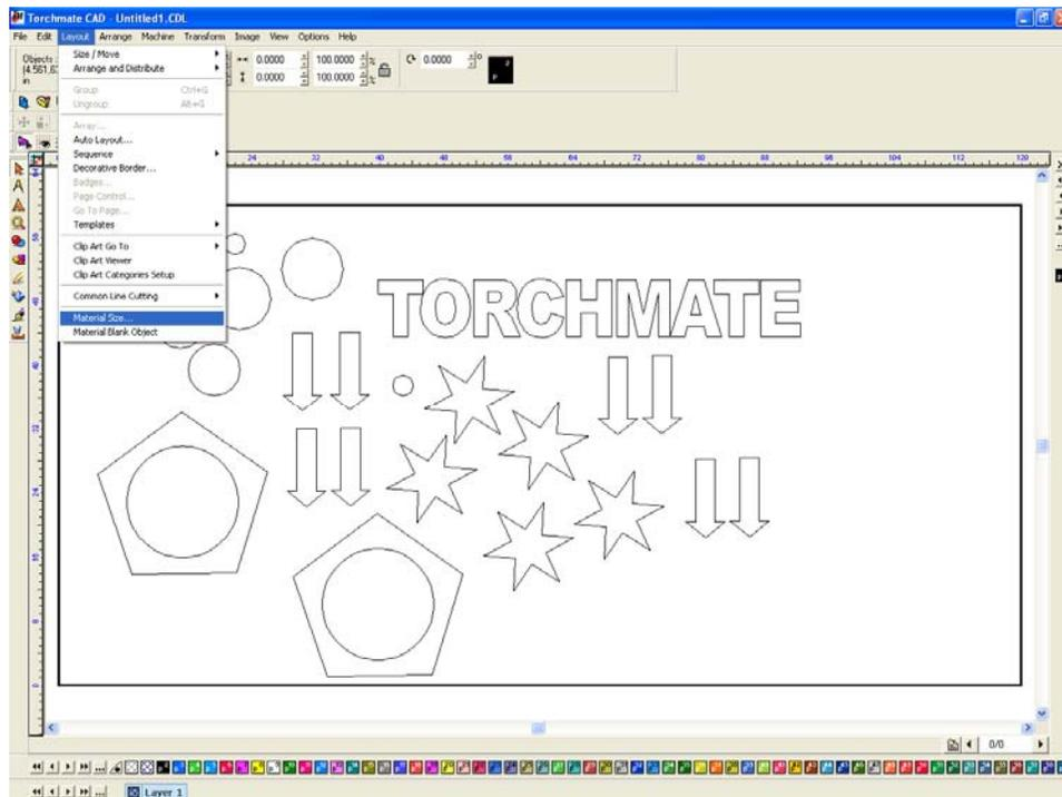
In the 'Material Size' window found in the 'Layout' menu the size and orientation of the work area can be defined.
