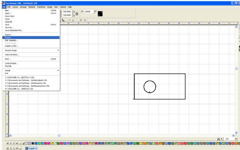
Ensure that the 'Save as type' is listed as 'DXF (Polyarc)'. Give the file a name and ensure that the location of where it is being saved is known. Select 'Export' and the file will now be able to be imported into the driver software to cut.
