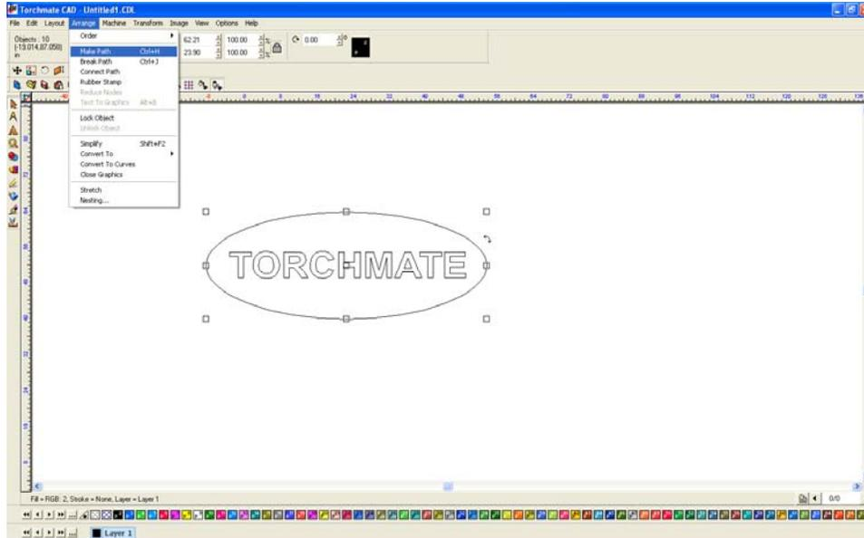
Once a part is done it is always a good idea to go to 'View' → 'Show Fill'. Show fill displays the part as the computer sees it, white space indicating scrap areas. When working with text letters with cutouts like 'O', 'B', 'A', etc. the cutout will fall out if it is not bridged.
