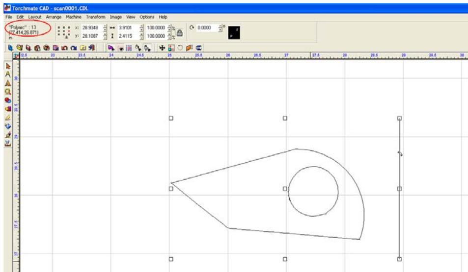
Some of the objects may just be double lines or scribbles, by moving parts away temporarily objects underneath can be seen.
