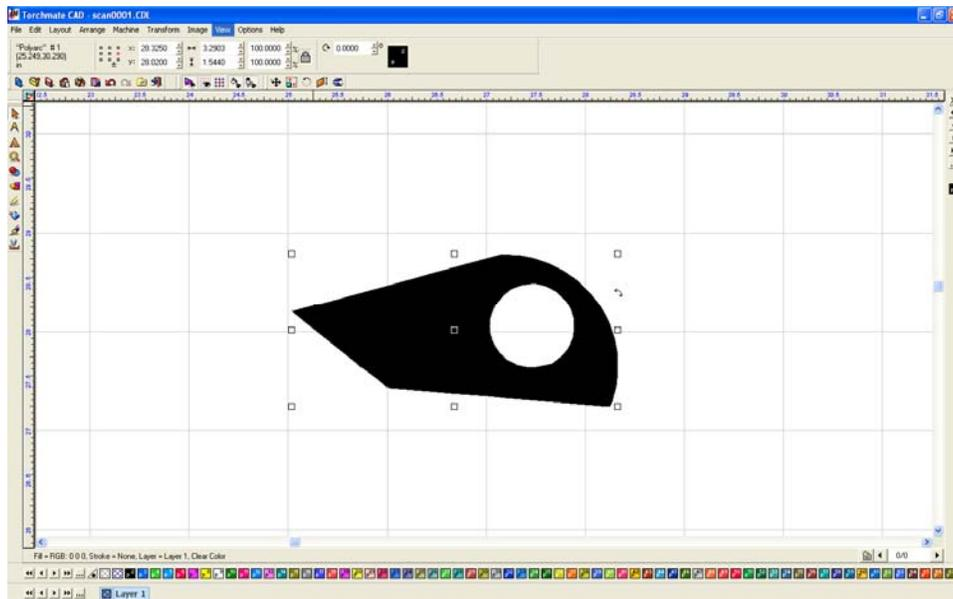
Node editing can be used to clean the object up. In this case selecting nodes that are unnecessary for the overall shape of the object.
