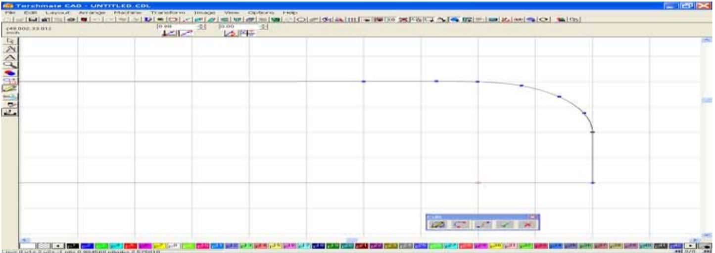
establish your two endpoints, and then choose the Line Segment Tool in the lower right corner of the Segment Palette to replace the segment with a straight line.
