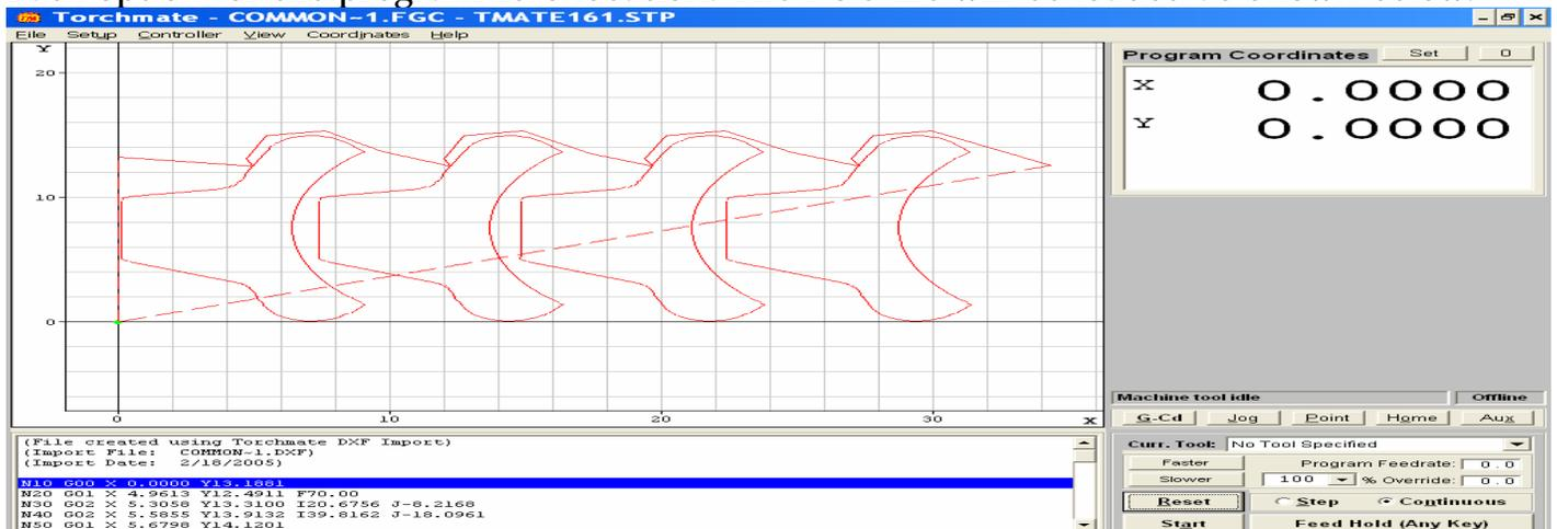
As you can see below, the first movement from the zero position is up along the Y axis, to the initial pierce point. The tool path then moves to the first part, cuts it, leads out to the next part, and continues to cut.
