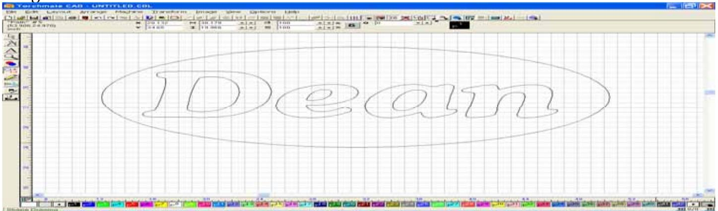
When the Show Fill tool is turned on, we can see that the letters are now part of the outside shape, but since the inside portions of the letters are not connected to the outside portions, they will fall out after the cutting has been performed.
