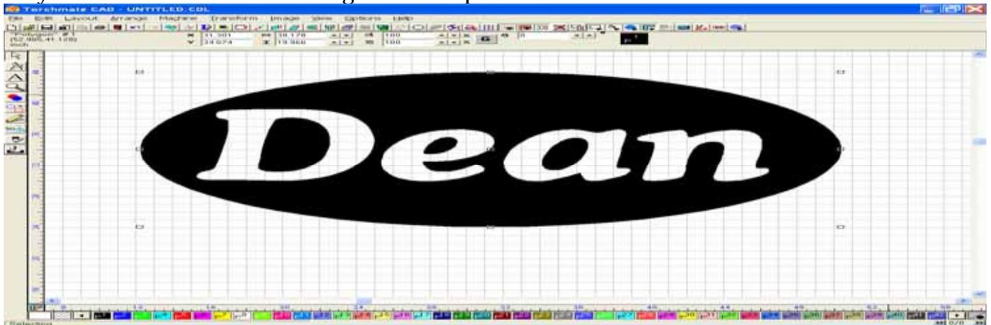
This picture shows an example of how the image would look after cutting, if the middle portion of the letters were not connected to the outside.
