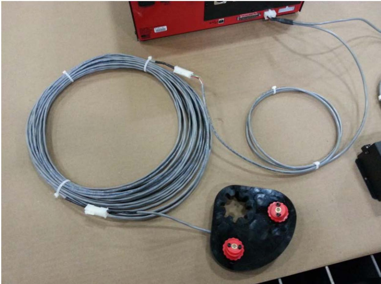
You should first start by plugging in your Interface Cable into the Output connection located on the back of Signal Generator.
