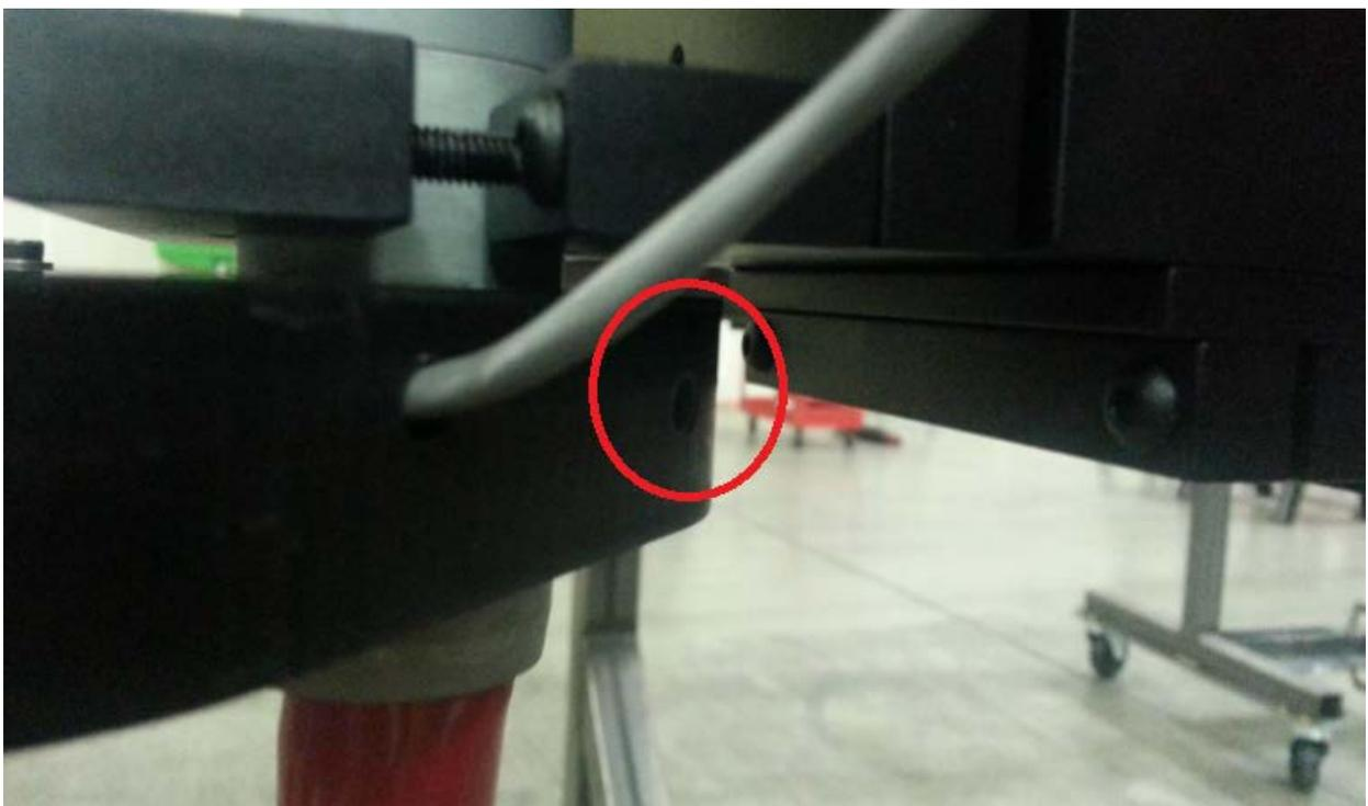
Now you can lead your wires through the cable carrier and connect it to the Interface Cable. Now all we need to do is set it up in the software.
