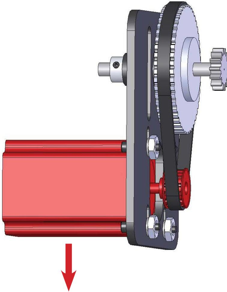
Belts should be adjusted hand tight. Ensure that there is no slop or backlash between the two pulleys.
