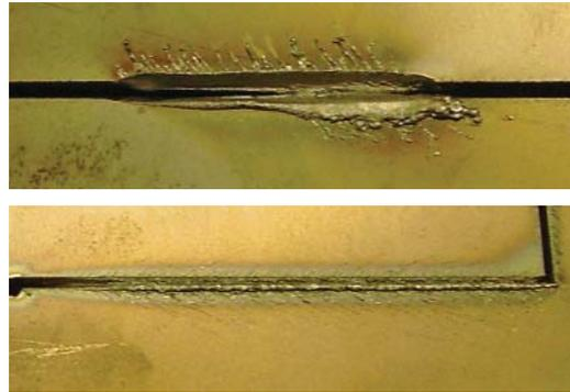
Instances where the metal was not fully cut indicate a few different problems. If the ground clamp was not properly attached to the material this can happen. A similar cut can happen if there was a drop in air pressure, moisture in the air line, or a drop in power. A third cause is if the torch contacts the material, most plasma cutters will go into a low power mode when this happens causing the cut not to penetrate all the way.
