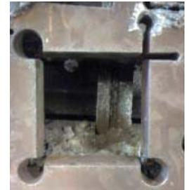
In the process to create a plasma arc for cutting the gas must be shaped into a vortex. Because of this an arc will have a direction of rotation. This will cause one side of the cut to have more bevel than the other. To ensure that the best bevel is on the part, proper direction of travel is necessary.
