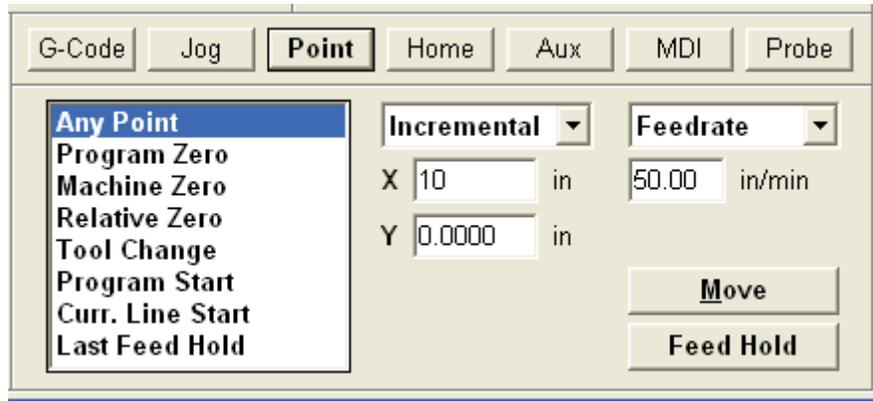
To move the table a certain distance go to the point menu and type in the desired distance to move. Measure how far the table actually moves. Using those two numbers and the current gear ratio a corrected gear ratio can be found. To find the current gear ratio and to change it go to “Configuration” ► “Machine” ► “Mechanics”
