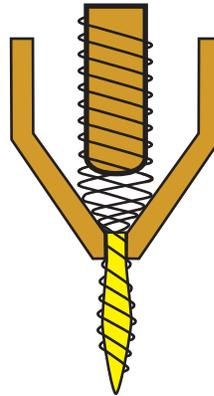
Consumables if not replaced regularly can cause bevel. If a tip wears out or slag builds on it the air flow is redirected in ways that can cause random bevel and inconsistent cut quality. Always check consumables when troubleshooting bevel.
