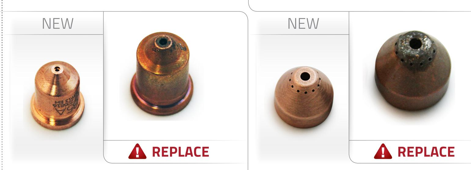
The shield cap orifice should be round and **smooth**. Because it is close to the work piece, it can suffer from spatter, and nicks. You can clean it with a non-metallic kitchen abrasive pad [don't use sandpaper], if it is not badly **burned**, dented, or cracked around the orifice. When you remove the shield cap, check the O-ring (if present) and its lubrication. S
