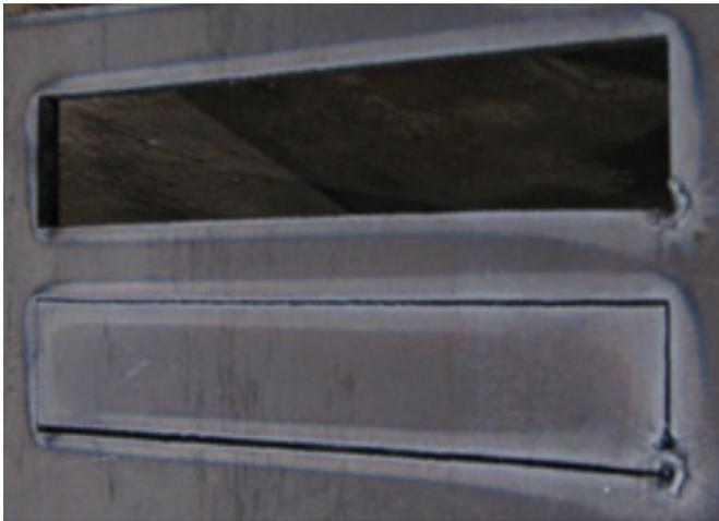
When the machine begins to move before a pierce is completed the cut will not complete. In this case the dwell time or pierce delay must be adjusted to allow for enough time to pierce the material.
