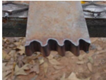
Corners can also have a bit more bevel than a normal cut. This is caused when the machine slows down to make the direction change. This can be minimized by adjusting ramping rates and start stop values. It is also possible in some cases to use a lower amperage to allow for slower travel speeds. This reduces the amount of slowdown through corners.
