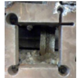
The direction of cuts are referred to as “conventional” and “climbing”. In a conventional cut the torch will go counter-clockwise on outside cuts and clockwise on inside cuts. A climbing cut is the opposite. For plasma the best bevel is achieved by using a climbing cut. Basically the best cut being to the right of the direction of travel.
