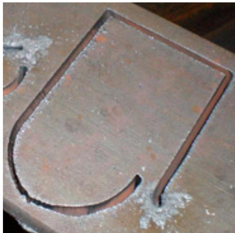
A cut where the path does not return to the start point indicates mechanical slipping or binding. In some cases it will be clear which axis is losing position. Examine the particular axis for loose set screws, loose belts, or physical obstructions.
