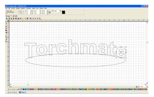
The next step is to rotate each letter. When a letter is selected there are nine boxes around the part as well as a small rotate tab, click on that and as the mouse is moved the letter will rotate.
