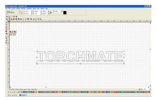
Be sure to turn on show fill once all editing is done to ensure that the CAD software is interpreting the drawing as it should be cut.
