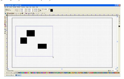
When selecting multiple objects it can sometimes become ambiguous as to which ones are selected and which are not. In Torchmate CAD there is a feature that when enabled highlights each selected object a certain color. This allows for easy identification of selected objects. To enable this feature go to 'Options' \(\rightarrow\)'Torchmate Setup' \(\rightarrow\)'Selection Tool Settings'.
