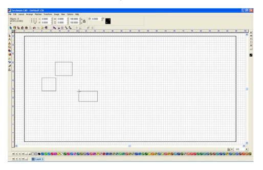
Multiple objects can be selected as well, the simplest way to do this is to click and drag with the 'Selection Tool' around the objects that are to be selected. Multiple objects can also be selected by using the 'Shift' key. With this method begin by selecting one object then hold down 'Shift' on the keyboard; click on another object both objects will now be selected. This method also works in reverse for unselecting a single object when multiple objects are selected.
