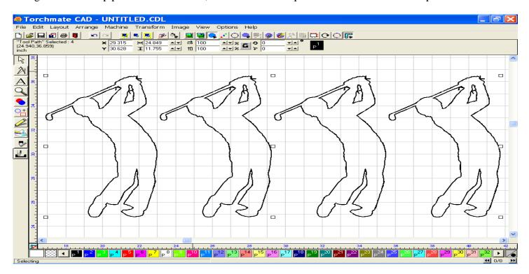
Use the Tool Path Viewer located in the View menu to see the sequence of cuts to be made. Click on Show Order to see the sequences.
