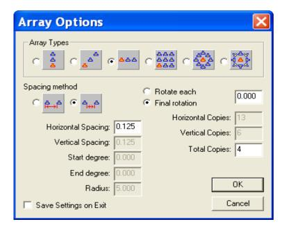
By using the specified field above, three additional copies were made, spaced horizontally.
