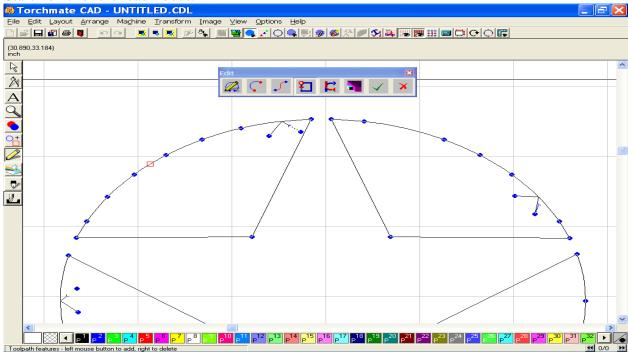
As you can see in the image below, the Start Point has be moved to reflect the change. Before moving to a new section to make changes, click on the green checkmark in the toolbar to complete the current changes.
