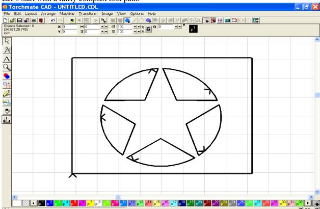
Double click the tool path to expose the nodes that make up the path. When the nodes are exposed, this toolbar will also appear. The tool fourth from the left is the Start Point tool, and can be used in the following examples to change the start point position in your image.
