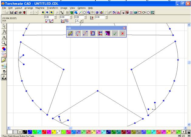
In the example below the lead position was changed, however when I made a change to a subsequent area, the first lead in returned to its original position.
