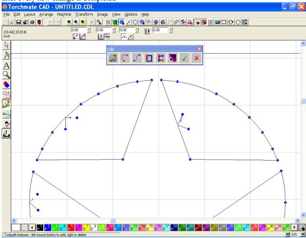
The Lead In/Out tool works similarly to the Start Point, except that it will only change one of the leads at a time, and will usually move the corresponding leads upon making new changes.
