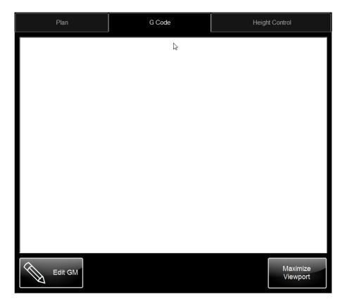
The G Code view is a text viewer which shows the file contents of the selected job. The g code view can be accessed by clicking on the G Code tab at the top of the Job View panel. Since a g code file is just a text file that only contains valid g codes, the g code view is essentially just a text viewer. When a job is running the currently executed g code will be highlighted in blue.
