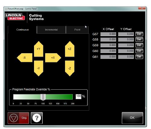
simply saving machine locations that are important for your application. The Fixture Offset utility provides a list of the available offsets and a method of setting the offsets for use in jobs.
