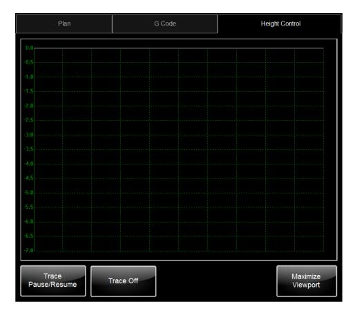
The Height Control view is a graph which displays the position of the Z axis. The height control view can be accessed by clicking the Height Control tab at the top of the Job View panel. The height control view is a good tool for diagnosing and observing the behavior of IHS sequences as well as how the AVHC is reacting to the material.
