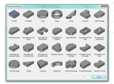
The shape browser displays all of the available shapes. To create a shape, select a template by clicking the image of the shape and then press the OK button to open the Shape Dimensions wizard.
