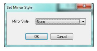
The mirror feature allows the selected job to be mirrored about the X, Y or both axis. Pressing the Mirror button will open up the Select Mirror dialogue box. Select the desired axis to mirror the job about. A mirror can only be applied when a job is not in progress (must be in a *reset* state). The mirror will be applied immediately after pressing the OK button on the Select Mirror dialogue box.
