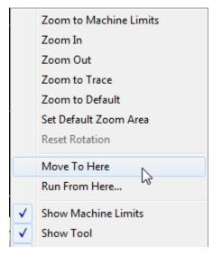
Click on any of the Zoom options to zoom in and out of the plan view. Clicking the 'Move to Here' option will cause the machine to jog the tool to the position on the machine that corresponds to the mouse curser. Learn more about the 'Move to Here' feature in the Tips and Tricks section of this manual.
