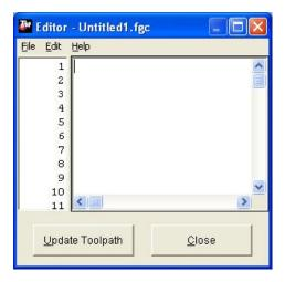
G-Code file names have an "FGC" extension by default. You can change the extension on the Files panel of the Configuration dialog box. Other common extensions used in the industry are "NC", "TAP" and "CNC."
