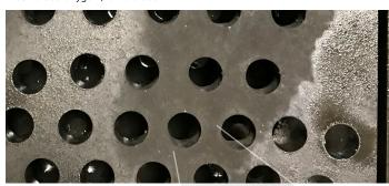
Secondary clearing gas steers the molten steel down the pierce hole without adhering to vs. the wall and exiting.
