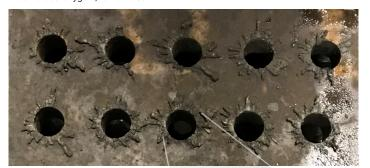
Dross is deposited — on the cut edge and spatter onto the top surface during the pierce.
